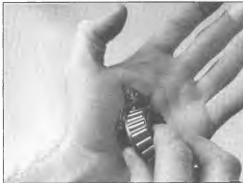
5.20 Work the grease completely into the rollers
