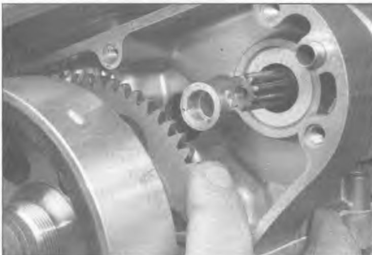
28.18 Check the starter clutch won't turn in a counterclockwise direction, but freewheels clockwise
