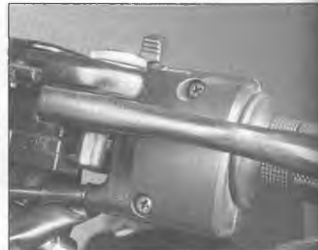
11.3a Remove the choke cable/switch housing screws . . .
