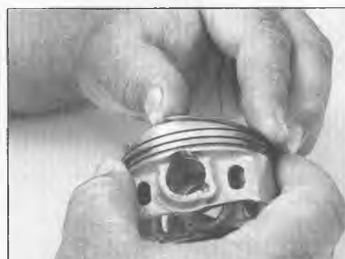
15.11a Install the second (middle) ring into the middle groove in the piston
