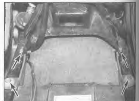
2.6a Remove the bolts (upper arrows); to remove the inlet duct, remove the screws (lower arrows)
