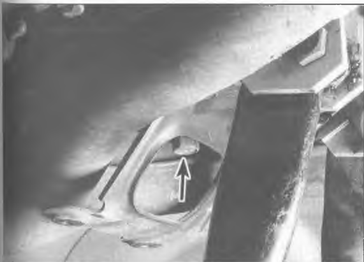
13.6 To detach the exhaust pipe, remove the two bolts (arrow - only one bolt visible in this photo)
