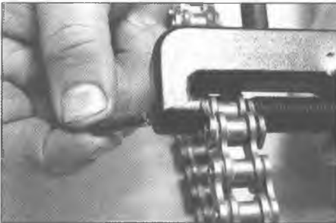
8.2 . . . withdraw the pin, remove the tool . . .
