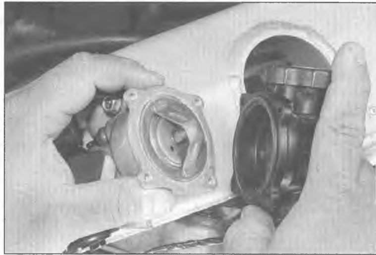
6.5 Remove the thermostat cover
