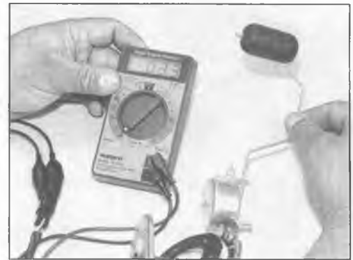
17.21 Measure the resistance of the fuel level sensor at the empty and full positions
