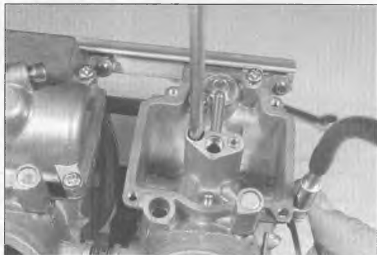
7.9a Unscrew the pilot jet ...
