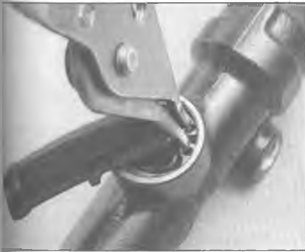
6.8a Remove the snap-ring that secures the fluid inlet fitting
