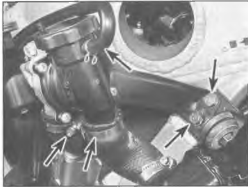
7.4 Loosen the hose clamps and disconnect the hoses, then remove the bolts (arrows)
