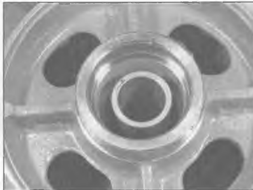
13.31b . . . and install the spacer in the hub
