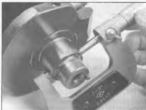
25.13 Measure the diameter of each crankshaft journal
