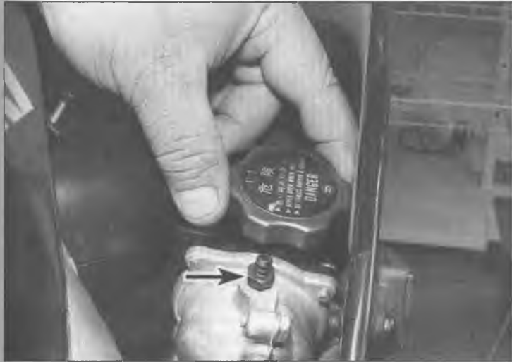
23.6 Turn the cap slowly to the first stop and allow all pressure to escape before removing it
