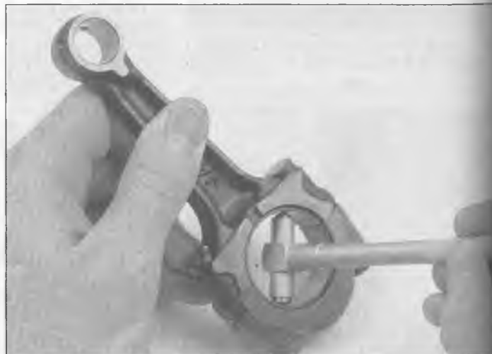
26.20b Measure the diameter of the connecting rod with a telescoping gauge, then measure the gauge
