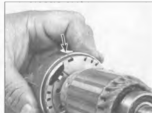
28.13c Make sure the notch in the brush plate is aligned with the notch in the armature housing
