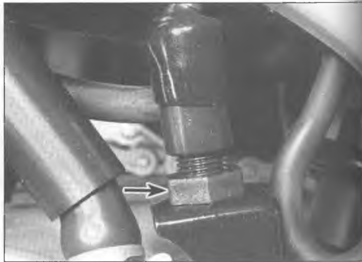
14.11 Back off the adjuster nut (arrow) and unscrew the switch from its bracket
