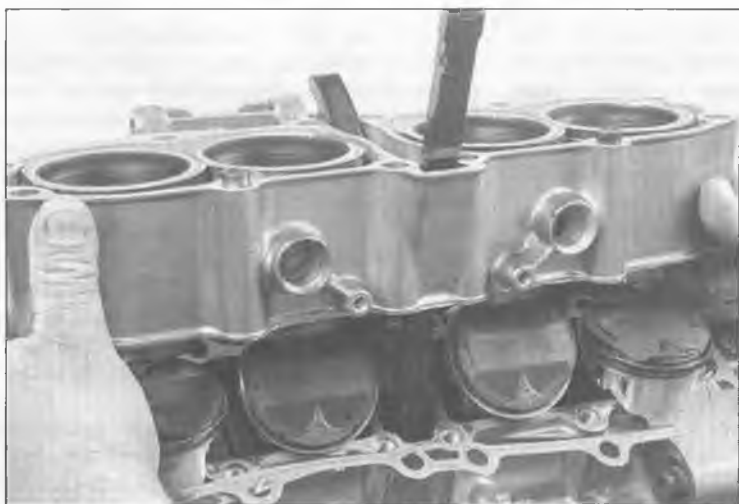
13.3c To remove the cylinder block, lift it straight up off the pistons
