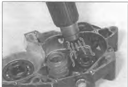
5.13 Using a localised heat source to aid bearing removal
