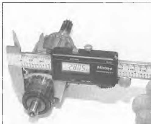
28.7 Check the commutator for cracks and discoloring, then measure its diameter
