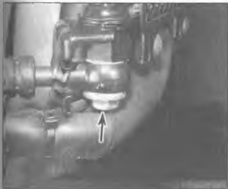
11.3 Remove the banjo bolts (arrow); discard the old sealing washers
