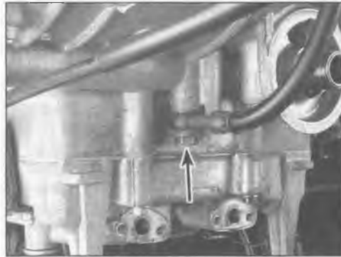
5.9b . . . and this banjo bolt (arrowed) from the crankcase
