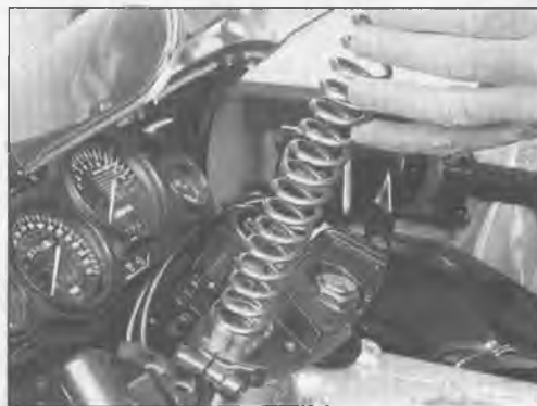
25.24e Remove the fork spring and remember which end faces down (the slightly tapered end)
