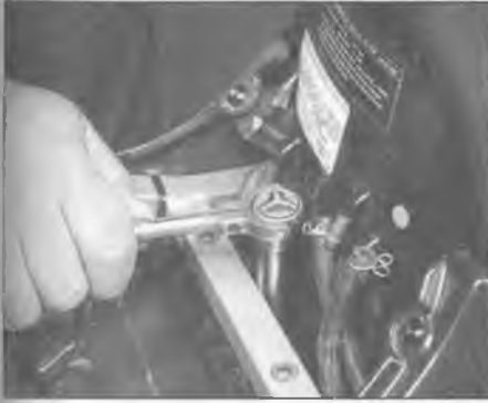
2.6b Remove the bolt that's located just underneath and ahead of this frame crossmember
