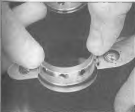
25.18 Make sure the tabs on the bearing inserts fit into the notches in the crank web
