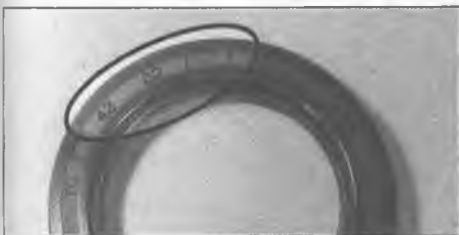
6.2 These oil seal markings indicate inside diameter, outside diameter and seal thickness
