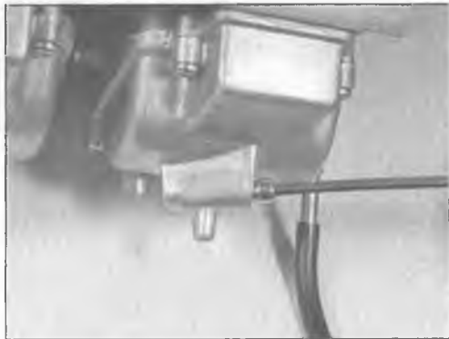
9.2a Loosen the float chamber drain screw
