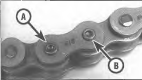
8.9 Pin end correctly riveted (A), pin end unriveted (B)
