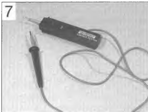
7 Battery-powered continuity tester
