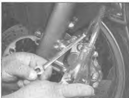
8.7 To bleed the brakes you need a box wrench, clear tubing and a container half-filled with brake fluid.
