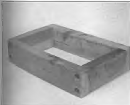
6.3 Construct an engine stand with short lengths of 2x4s and lag bolts or nails
