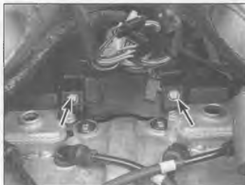
5.15a To detach the center heat guard, remove these two bolts (arrowed)
