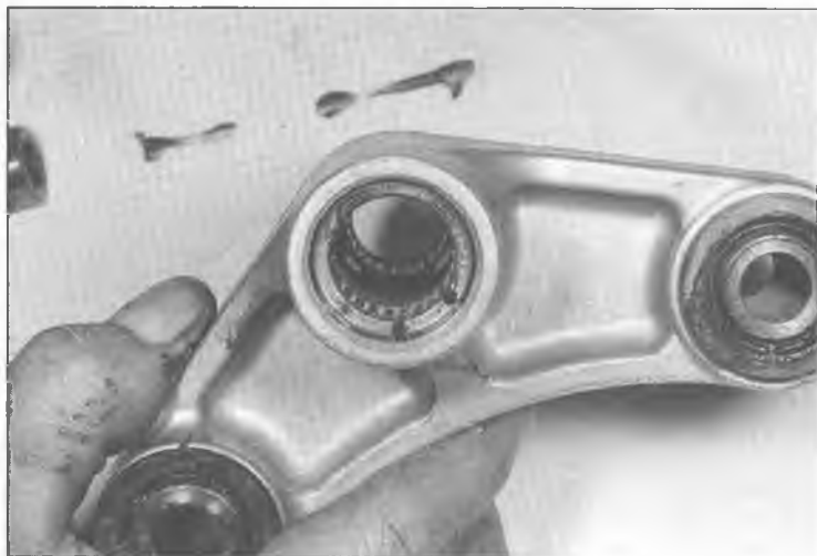
7.5 Inspect the needle bearings inside the rocker arm
