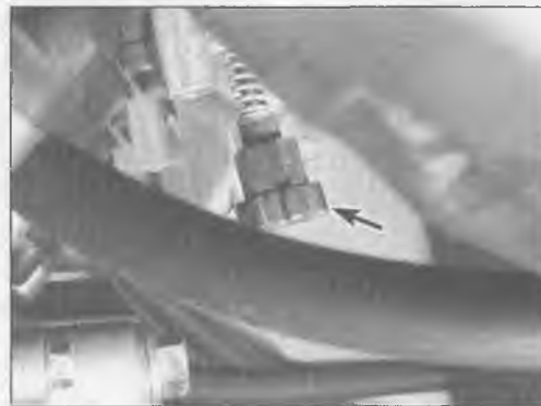
6.19a On D models, the idle speed screw (arrow) is underneath the carburetors
