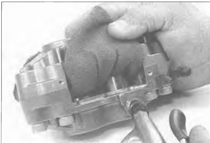
2.8 Place rags in the brake pad cavity and apply a blast of compressed air to break the pistons loose
