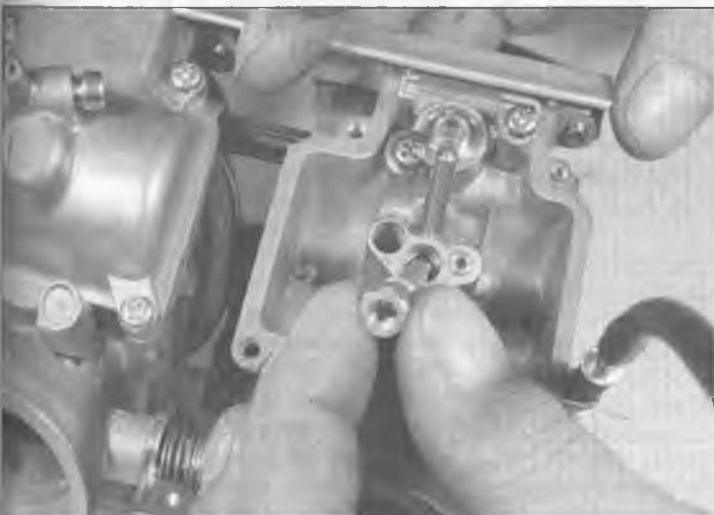
7.8 Unscrew the needle jet holder
