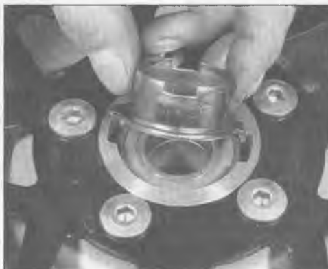
13.3b . . . to remove the speedometer drive
