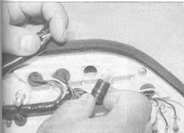
18.2a To remove a bulb holder from the instrument, simply pull the holder straight out
