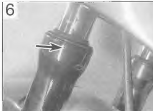
Inspect the area around the fork dust seal for oil leakage (arrow)
