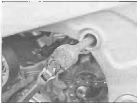
5.18b Use the same technique to remove the upper rear engine mounting bolt
