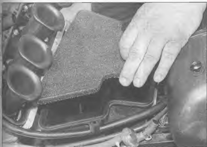
14.3a Removing the air filter on a D model
