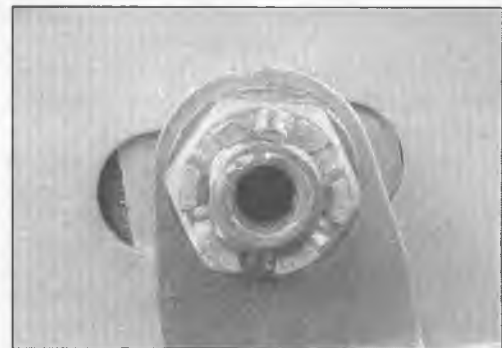
2.11 When the chain is adjusted, make sure the marks on the swingarm correspond on each side
