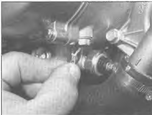
19.2b Disconnect the wire, turn on the ignition main (key) switch and ground the end of the wire
