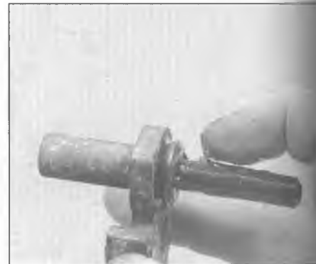
2.28 Apply a thin coat of the specified grease to the slider pins on the caliper bracket
