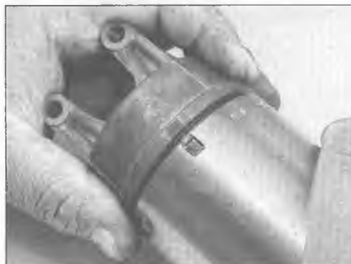
28.2a Mark the relationship of the end covers to the armature housing
