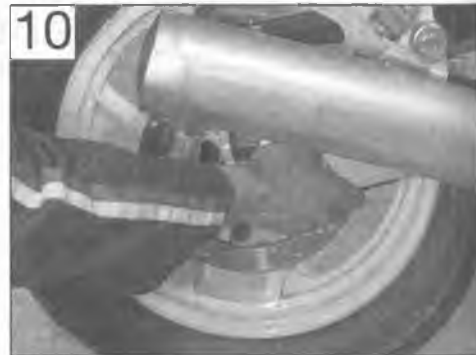
10 Grasp the swingarm at the ends to check for play in its pivot bearings
