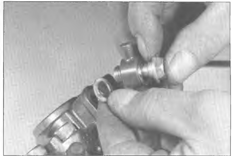
2.2b Remove and discard the copper sealing washers on each side of the banjo fitting
