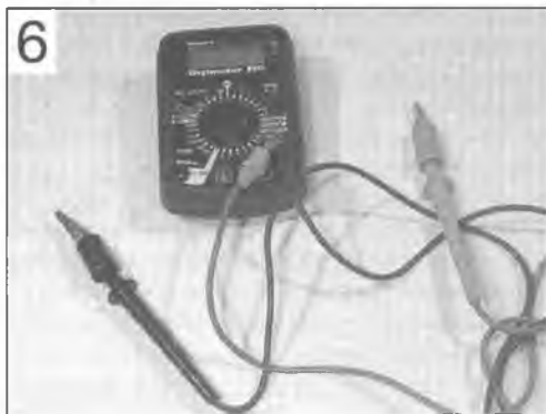
6 Digital multimeter can be used for all electrical tests
