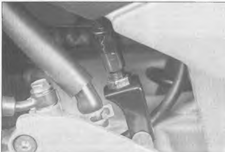
10.6 Hold the switch and turn the adjusting nut on the switch body until the brake light is activated
