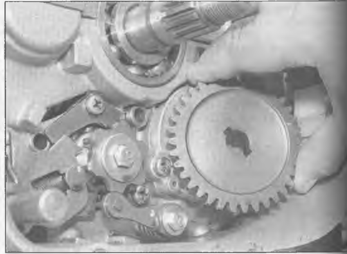
17.10 Remove the oil pump gear
