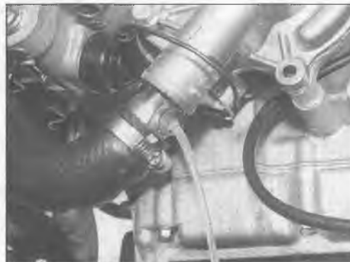
23.12 Remove the bolt from the water pump outlet pipe (hose disconnected from inlet pipe for clarity)
