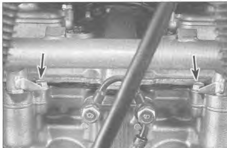
10.5 Loosen the clamp and detach the hose from the right end of the pipe, then remove the bolts (arrows) and pull the pipe ends out of the cylinder head
