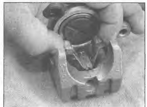
2.17e Remove the anti-rattle spring
