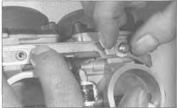
7.2b . . . and the three choke shaft screws . . .
