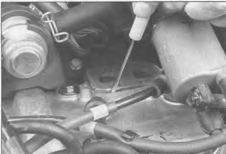
4.5a Remove the retaining bolts and the valve cover, then carefully pry the reed plate out of the cover
