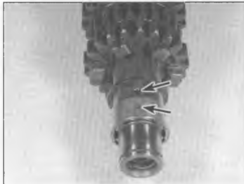
30.13c Be sure to align the bushing oil hole with the shaft oil hole (arrowed)
