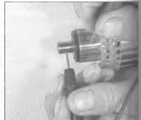
28.8b There should be no continuity between the commutator bars and the armature shaft
