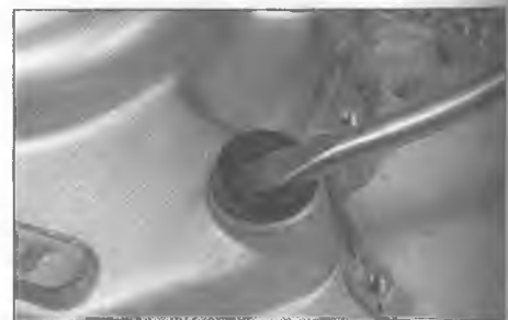
6.1 Prise out oil seals with a large flat-bladed screwdriver
