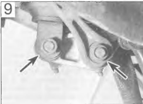
9 Worn suspension linkage pivots (arrows) are usually the cause of play in the rear suspension
