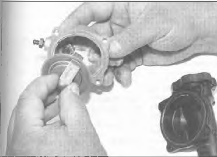
6.6a Remove the thermostat from the housing, noting how it's installed . . .
