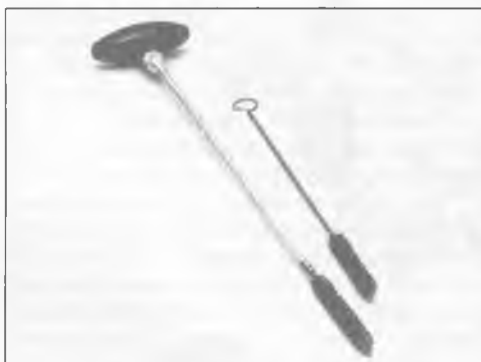
6.2a A selection of brushes is required for cleaning holes and passages in the engine components
