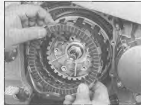
20.6 Remove the clutch friction and steel plates
