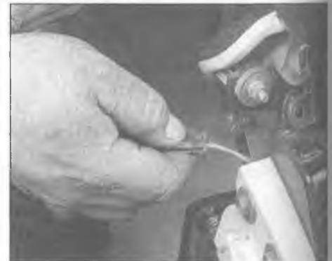
8.3f Before removing the side cover on E models, unplug the connector for the turn signal light
