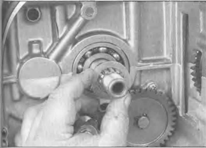
20.8g Remove the small washer
