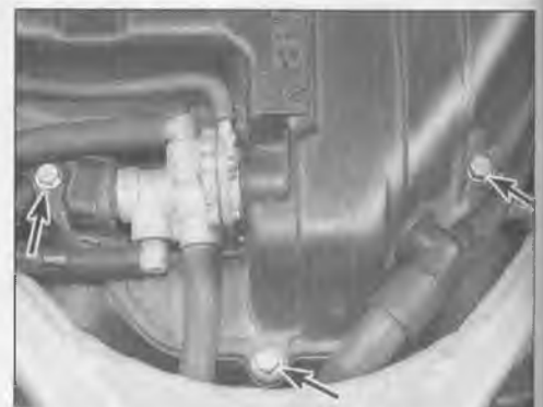
14.2c . . . and remove these bolts (arrows); to ensure proper reassembly, clearly label all hoses
