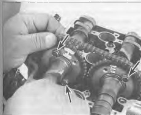
9.6a Label the camshaft sprockets and remove the three bolts (arrowed) you can see
