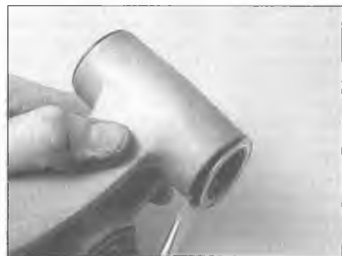
7.6c Pry out the dust seals from the rocker arm (shown) and the swing arm (not shown)
