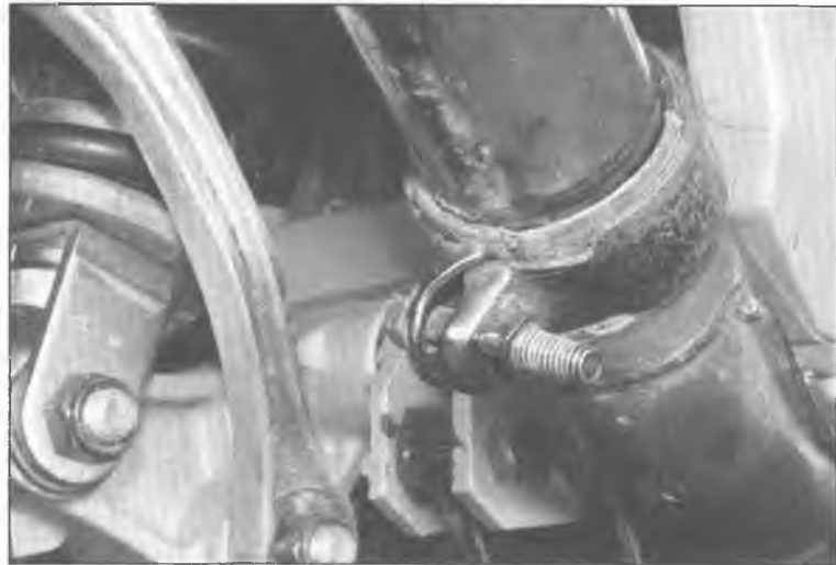
13.5 Loosen the muffler-to-exhaust pipe clamp bolt
