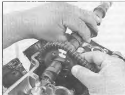
9.6b Slide the intake cam through the intake sprocket and remove it . . .
