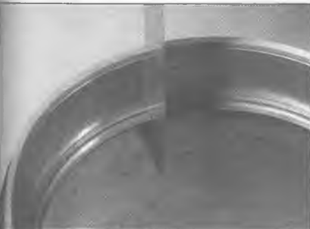
3.1 Feeler gauges are used for measuring small gaps and clearances - thickness is marked on one face of gauge
