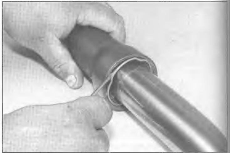
4.7 Pry the retainer ring out of the outer fork tube with a small screwdriver
