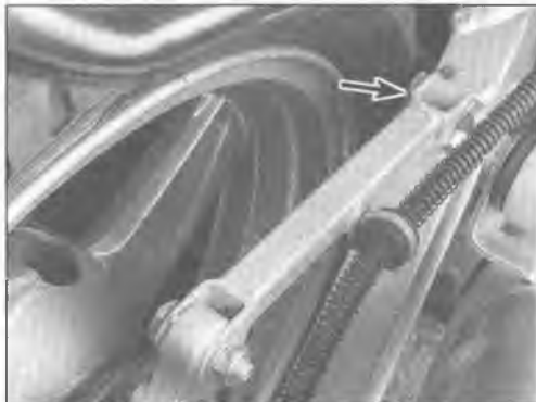
9.3 To disconnect the torque arm from the swingarm, remove this nut (arrow) and bolt
