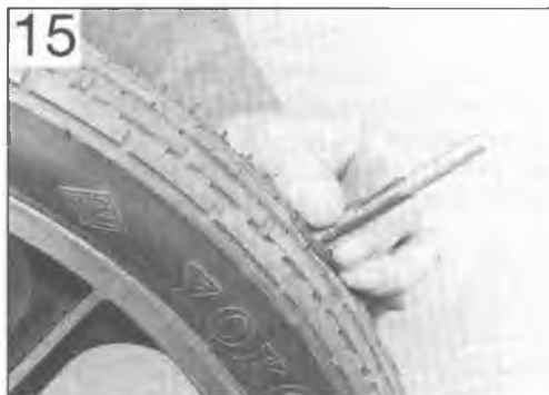
15 Checking the tyre tread depth
