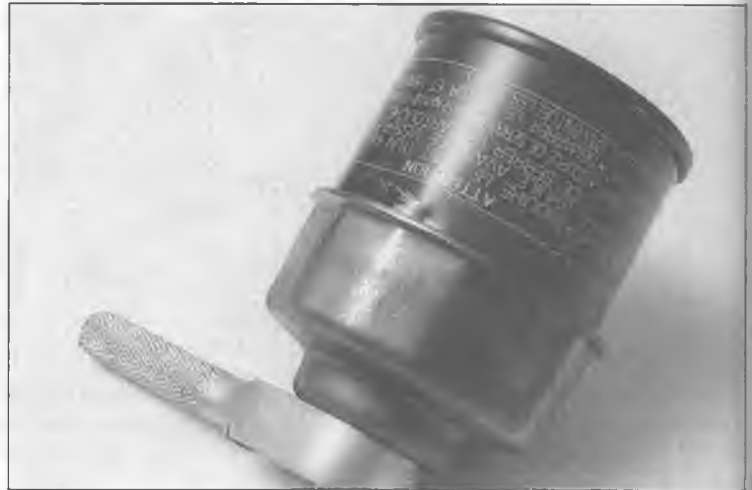
13.7b Properly engaged, the filter and filter wrench look like this (filter removed from bike for clarity)
