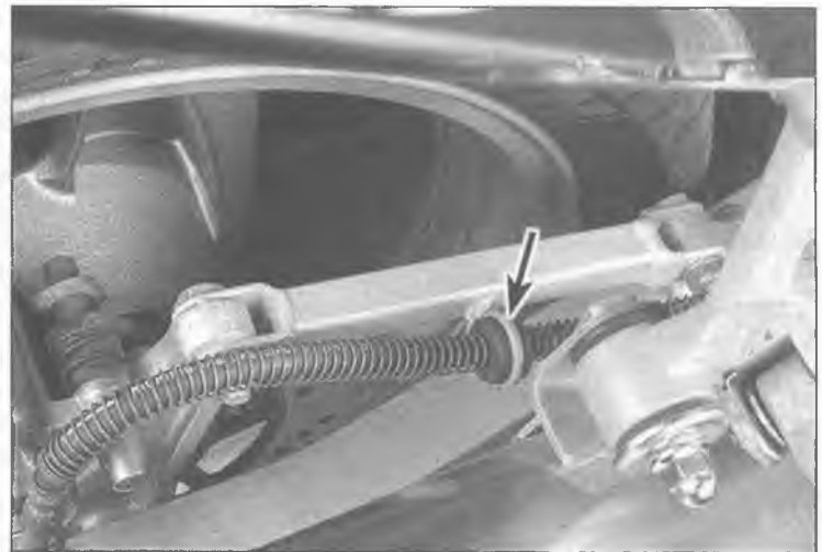
2.4b Separate the brake hose from its clip on the torque arm
