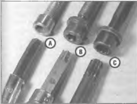
2.1 Internal hexagon/Allen (A), Torx (B) and splined (C) fasteners, with corresponding bits
