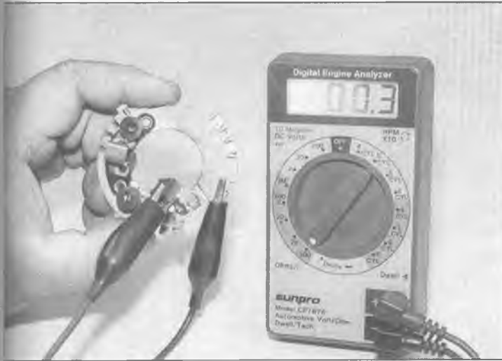
28.9 There should be virtually no resistance between the negative brush and the brush plate
