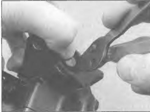
5.10a . . . then depress the piston and remove the snap-ring with a pair of snap-ring pliers
