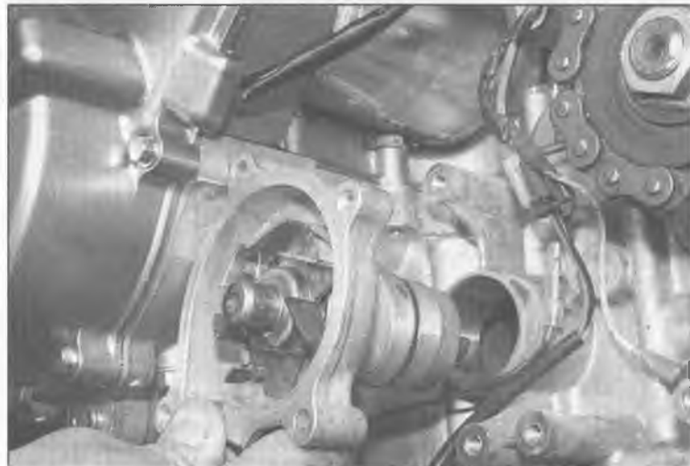
9.13 To remove the water pump assembly, pull it straight out of the engine
