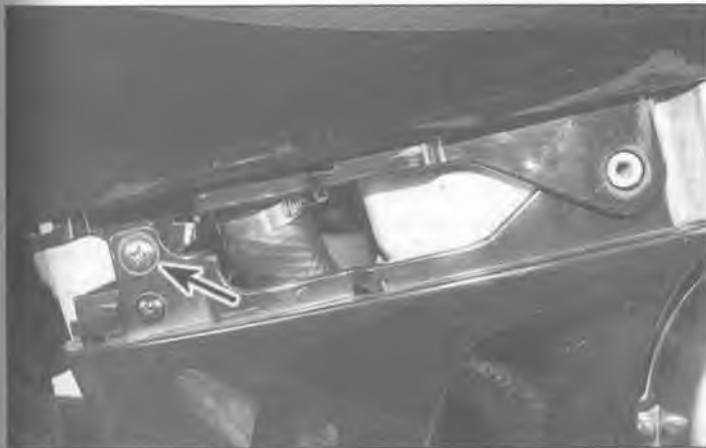
2.9 Remove the screws (arrow) that attach the lower fairing to the frame (E model shown)
