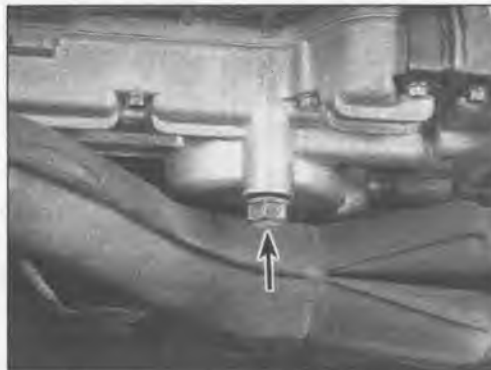
13.6 Remove the drain plug (arrow) from the engine and allow the oil to drain into a pan
