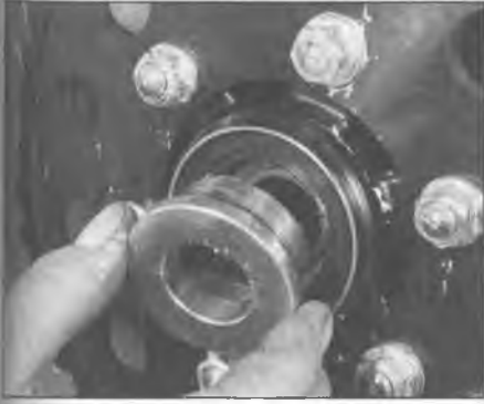
13.15a Remove the spacer . . .
