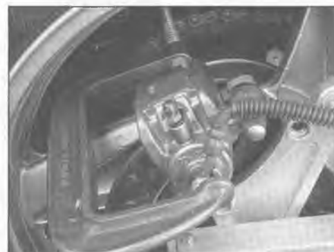
2.7 Tighten the clamp to push the piston into its bore so the caliper fits over the disc with the new pads
