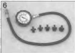
4 Cylinder compression gauge 5 Vacuum gauges (left) or manometer (right) 6 Oil pressure gauge
