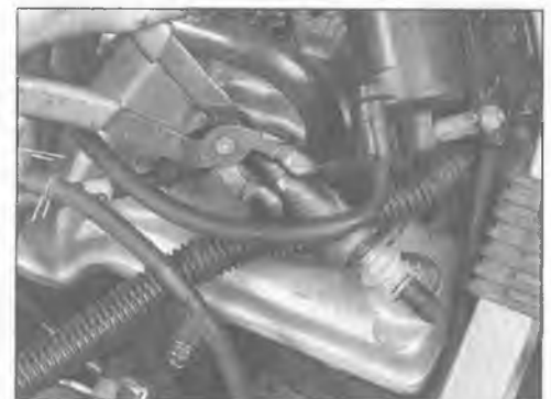
2.3 Ground (earth) a spark plug and operate the starter - bright blue sparks should be visible
