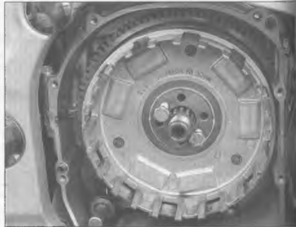
20.8d To separate the sleeve from the housing, install a couple of bolts as shown, screw them in and pull it out
