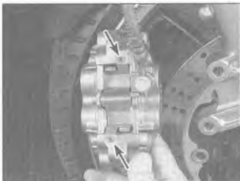
3.2 To get at the pads on either front caliper, remove the pad cover screws (arrows) and the cover
