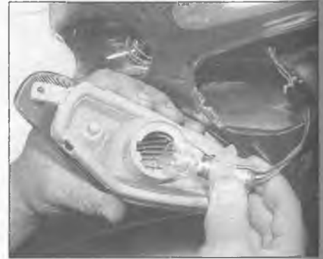
11.2a To remove a bulb holder from the front turn signal assembly, turn it counterclockwise and pull out
