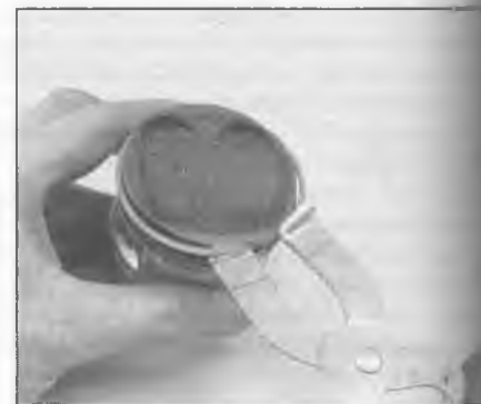
14.6 Remove the piston rings with a ring removal and installation tool
