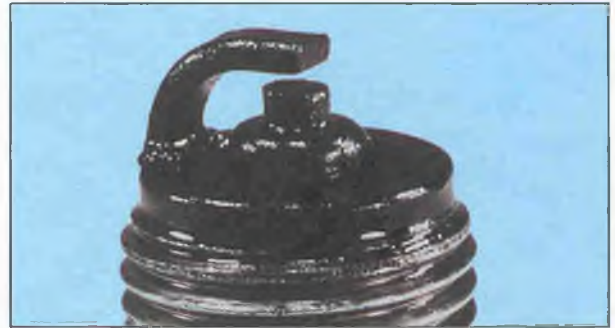
Oil fouling – Wet oily deposits leading to misfire and weak spark. Caused by oil leakage past piston rings or valve guides (4-stroke engine), or excess lubricant (2-stroke engine).
