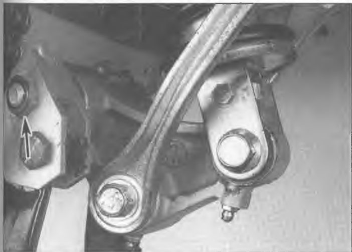
7.4 Remove the nut and bolt which attach the rocker arm to the frame (arrow)
