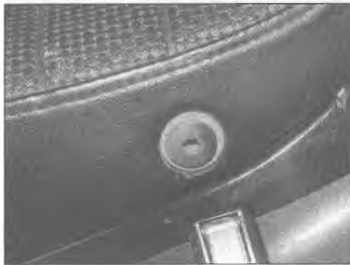
7.1 To remove the seat from a D model, remove the bolt from each side of the seat
