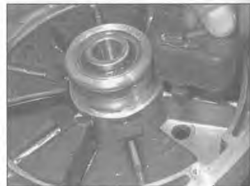
Cush drive rubbers dampen out transmission shocks
