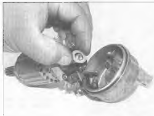
28.13b Don't forget to install this washer on the commutator shaft before inserting the shaft
