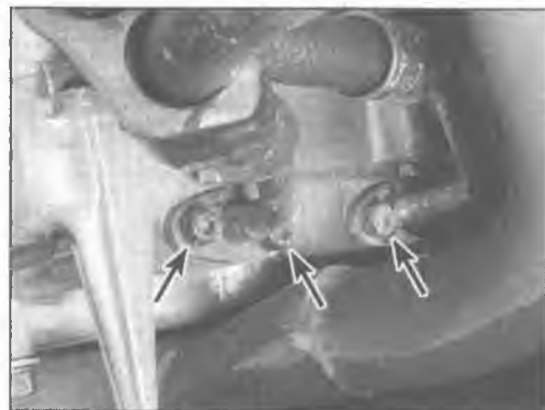
11.5 To detach the oil cooler hoses from the engine, remove these flange bolts (arrows)
