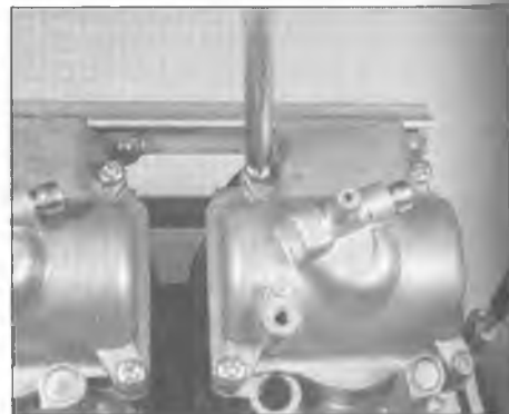
7.5a Remove the float chamber cover screws ...
