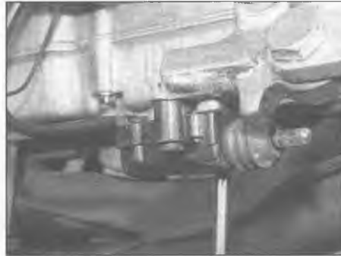
24.6 The sidestand switch is secured by two screws
