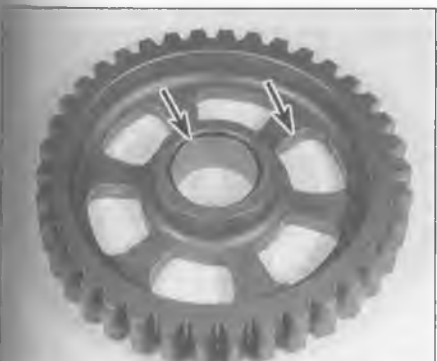
30.11 Replace the gear if the bushing (left arrow) is worn; also if the slot edges (right arrow) are rounded
