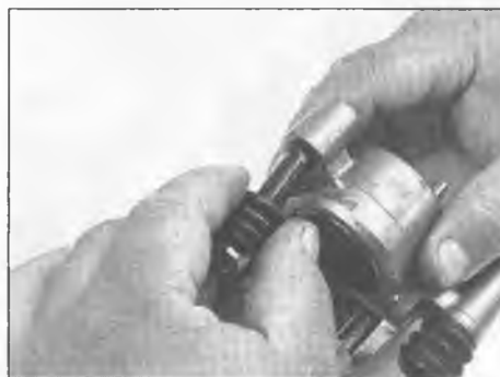
2.17d . . . and remove the slider pin boots
