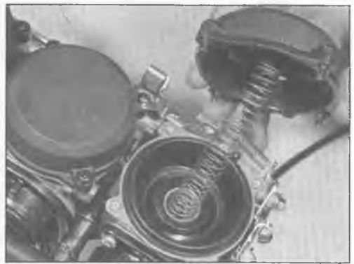
7.3c . . . lift off the cover and spring . . .
