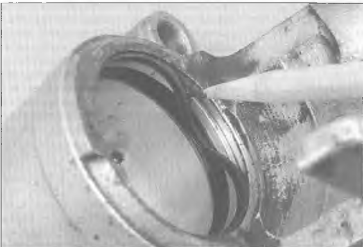
2.11 To avoid damage, use a pencil - or some other plastic or wooden tool - to remove the seals
