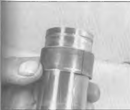
4.11c The outer tube guide bushing can now be removed by simply sliding it off
