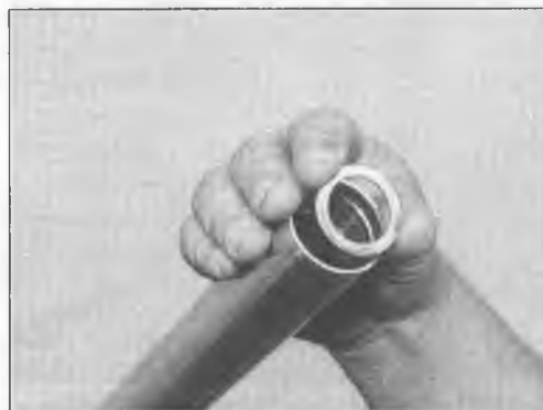
25.16d . . . and remove the spring seat (a magnet may be required to do this)
