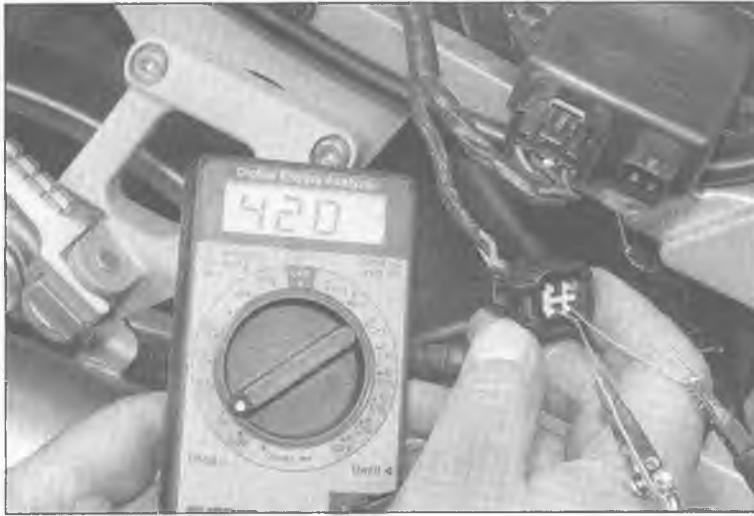
4.3 Measure the resistance across the two pickup coil terminals
