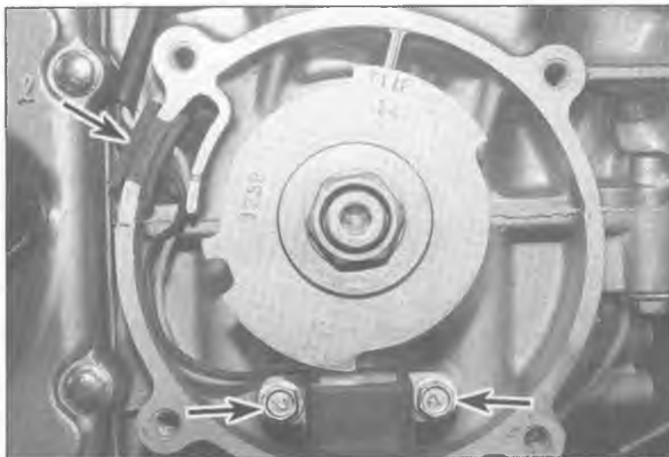
4.7 Remove the screws (arrows), pull the grommet (arrow) for the leads out of its notch in the case
