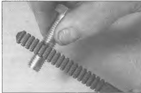
2.24 Using a thread restorer file
