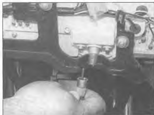
15.2b Unscrew the threaded ferrule and disconnect the speedometer cable from the speedometer
