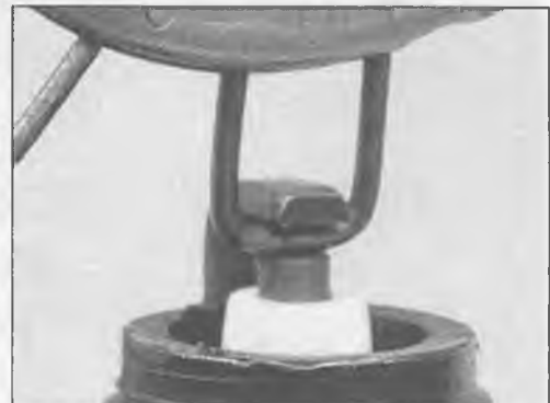
3.6a Spark plug manufacturers recommend using a wire-type gauge for checking the spark plug gap
