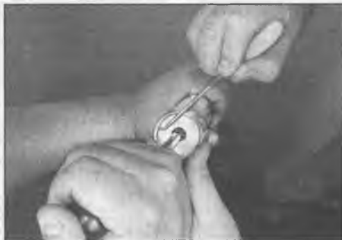
25.16a Push the top plug into the fork tube and remove the wire retaining ring, then remove the plug
