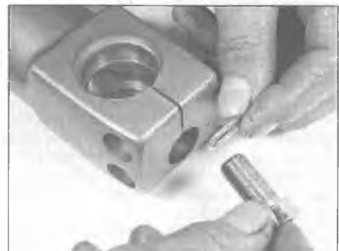
4.5c Remove and discard the old sealing washer
