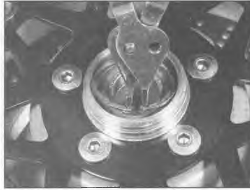
13.4c Remove the snap-ring from the right side of the wheel
