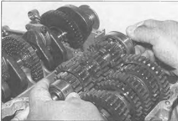
28.2 Once the crankcase has been separated, the transmission shafts can be lifted out
