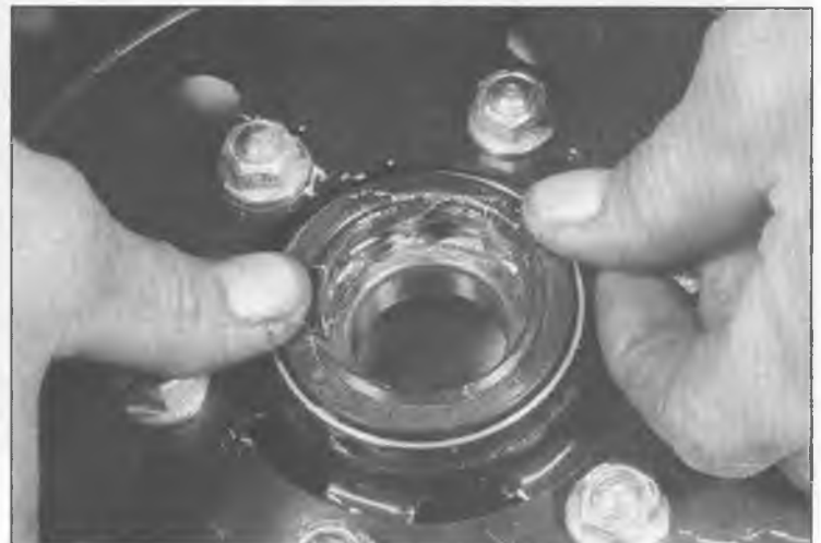
13.23 Press in the new grease seal
