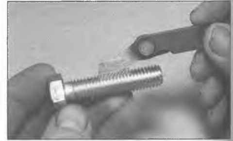
2.12 Using a thread gauge to measure pitch
