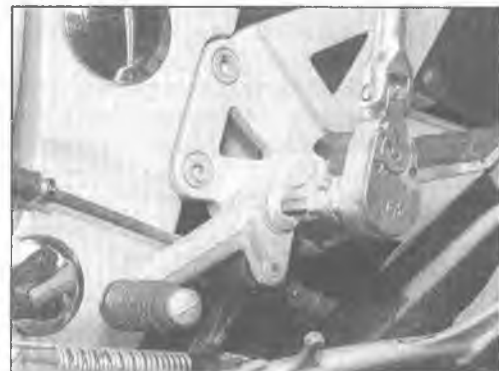
11.3 Unscrew the shift lever pivot bolt from the left footpeg bracket
