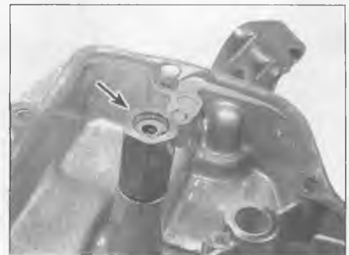
18.2a The oil pressure relief valve (arrowed) for the oil cooler and transmission is screwed to the oil pan
