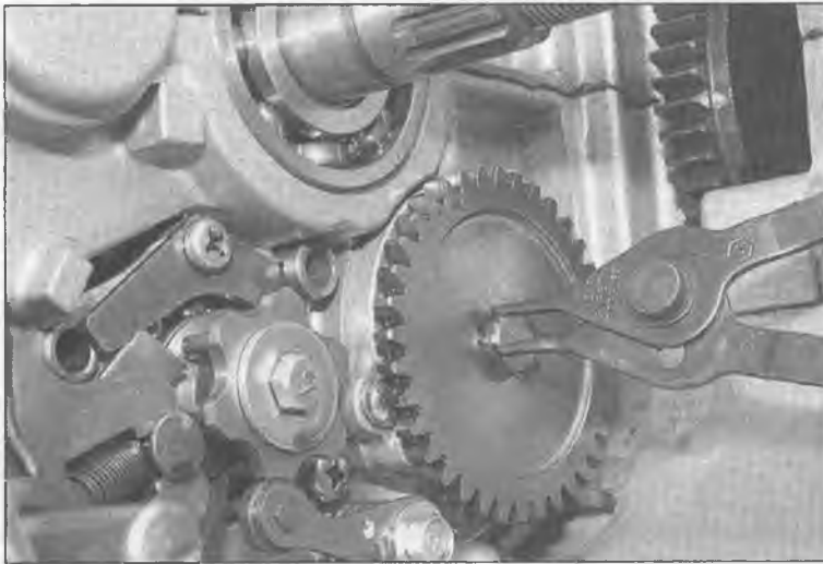
17.9 Remove the oil pump gear snap-ring
