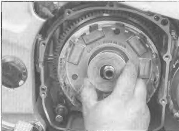
20.8c Remove the large washer
