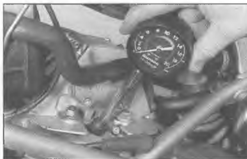
3.20 Using a rubber-cone type cylinder compression gauge
