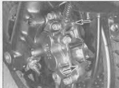
9.2a To gain access to the brake pads, remove these screws (arrows) and remove the pad spring
