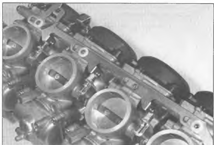
8.14b Be sure to reinstall the plastic washers on both sides of the shaft
