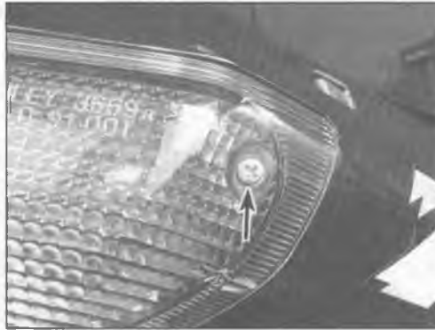
11.1b To detach a rear turn signal lens, remove this screw (E model shown)
