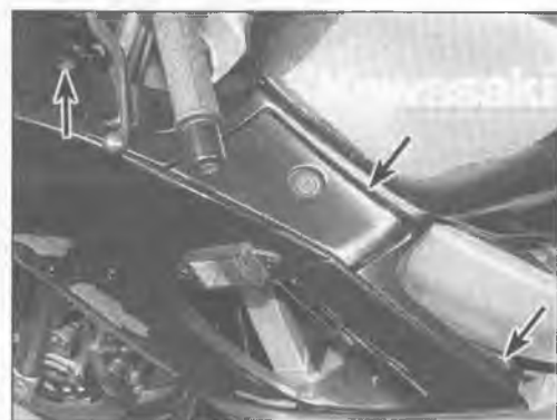
6.12a To remove the left trim panel on E models, remove these screws (arrows)
