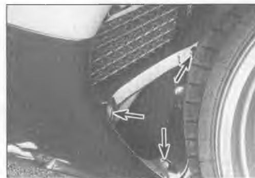
2.12 To detach the lower fairing halves from the front piece, remove these three screws (arrows)
