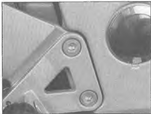
11.9 To remove the right footpeg and bracket from the frame, remove these two Allen head bolts
