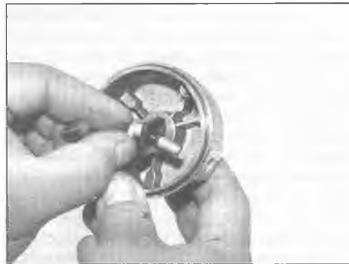
28.12a Install the terminal bolt in the rear end cover
