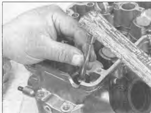
12.26 Using the handle of a hammer, an extension and a small socket, tap on the valve guide seals
