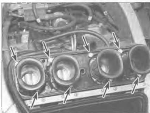
7.2e Intake boot mounting screws (arrows) (D models)
