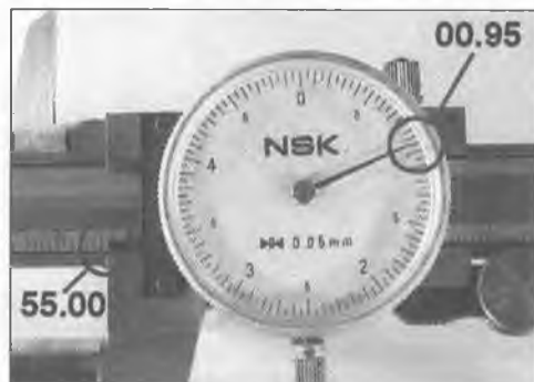
3.14 Vernier gauge reading of 55.95 mm
