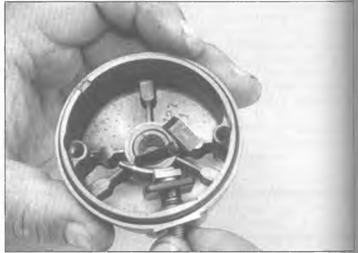
28.5 Remove the nut from the terminal bolt and push the bolt through the end cover
