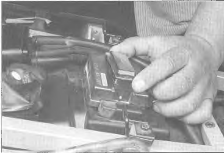
5.1a To get at the fuses inside the junction box, remove the plastic cover by pulling up on either end
