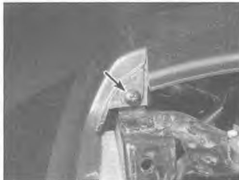
8.3e ... and this screw at the inner end of the panel (arrow)
