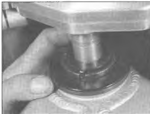
5.23 Install the lockwasher, making sure it engages the notches in the nut
