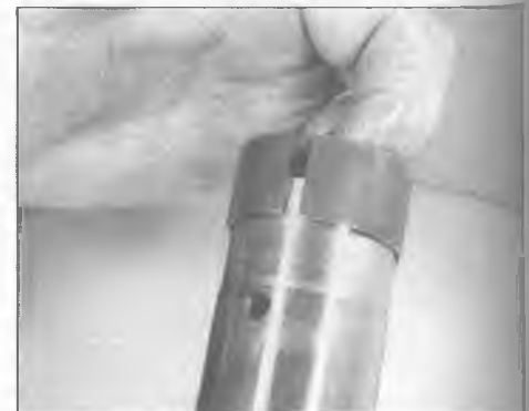
4.11b To remove the inner tube guide bushing, pry it apart at the slit and slide it off
