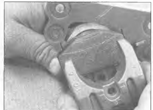
3.15 When installing the pad that fits against the piston, be sure it's properly engaged with the bracket
