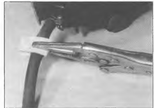
9.4 ... or thick card and self-locking grips
