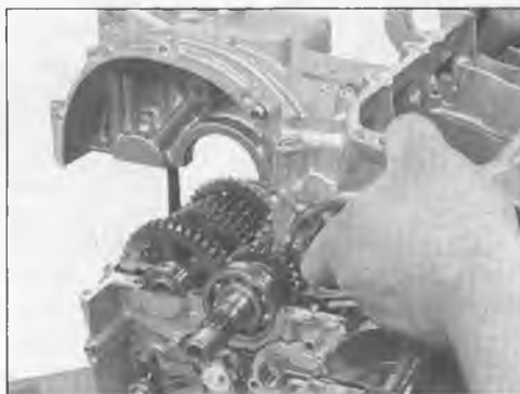
22.5a Separate the crankcase halves
