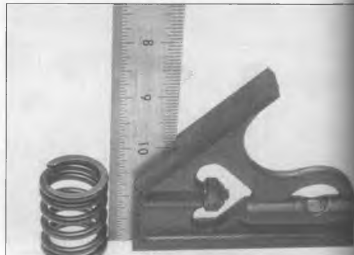
12.19b Checking the valve springs for squareness
