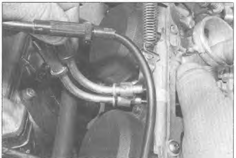
5.7c . . . then remove the elbow-shaped cable housings from their brackets on the carburetor
