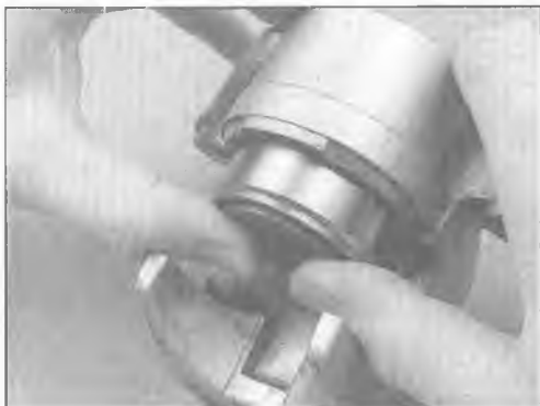
2.26 Bottom the piston in the caliper bore - make sure it goes in straight
