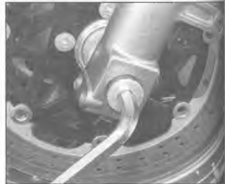
11.4b Remove the axle nut from the left slider
