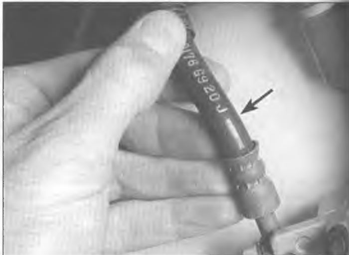
7.2 Flex the brake hoses and check for cracks, bulges and leaking fluid
