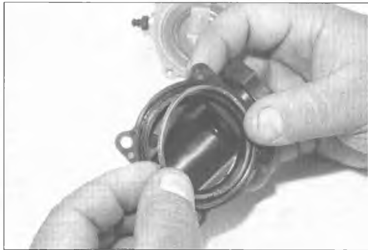
6.6b . . . and remove the O-ring from the cover
