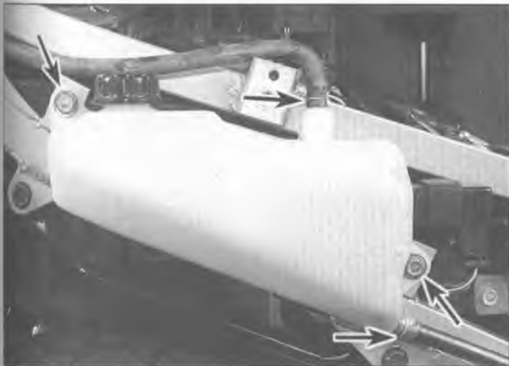
3.2 To detach the reservoir, disconnect the hoses, then remove the retaining bolts (arrows)
