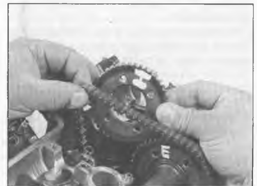
9.6c . . . then remove the intake cam sprocket
