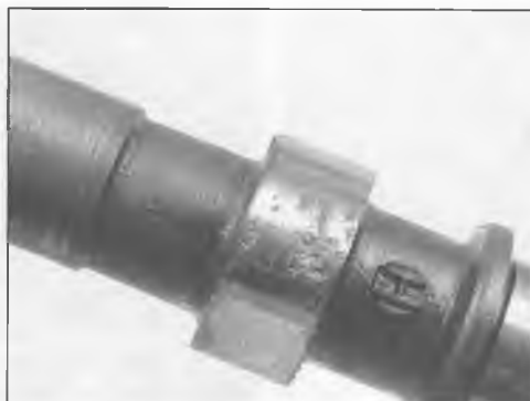
9.9a Check the lobes for wear - here's a good example of damage which requires replacement or repair
