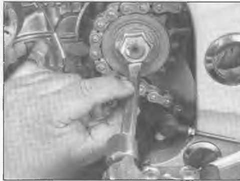
16.6a To remove the countershaft sprocket, flatten the folded-up sides of the lockwasher . . .
