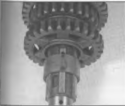
30.17d ... its bushing and fourth gear
