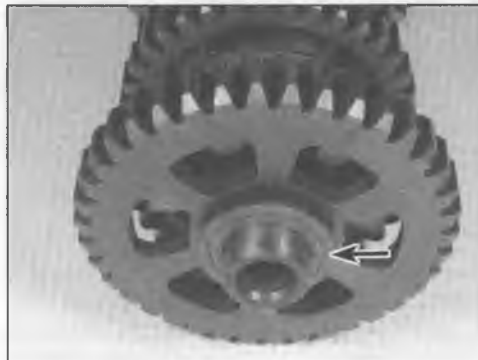
30.15 Remove the thrust washer (arrowed) and first gear
