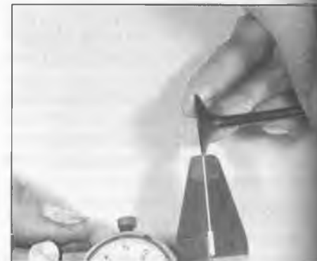
12.18c Measuring valve head margin thickness
