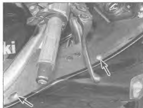
4.2d . . . and remove these screws (arrows) from the right side
