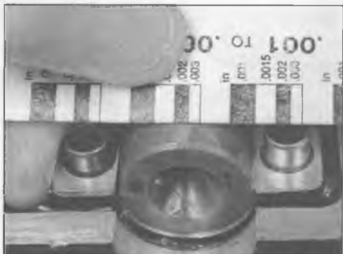
9.13a Compare the width of the crushed Plastigauge to the scale printed on the Plastigauge container
