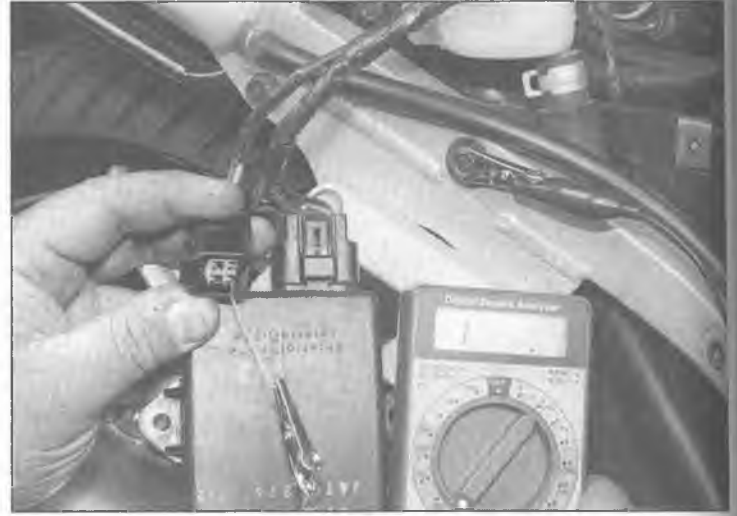
4.4 Measure the resistance between each pickup coil terminal and ground
