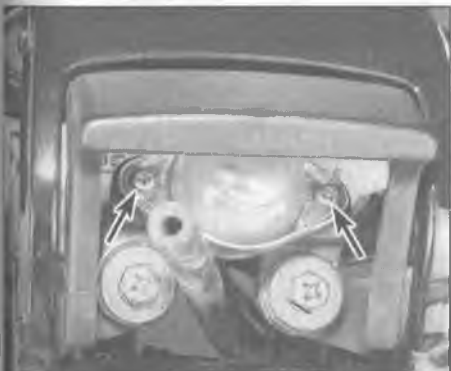
11.9 To remove the license plate light lens, remove these screws (arrows)
