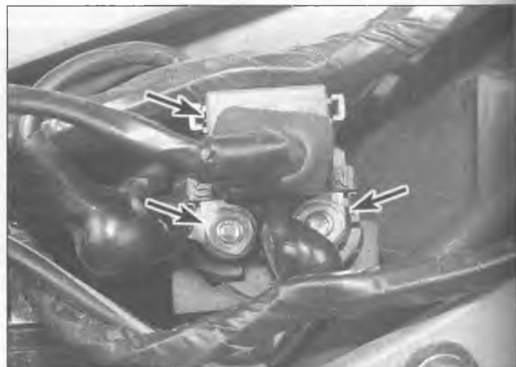
26.2 To remove the starter relay, remove the terminal nuts (lower arrows) and unplug the connector (upper arrow)
