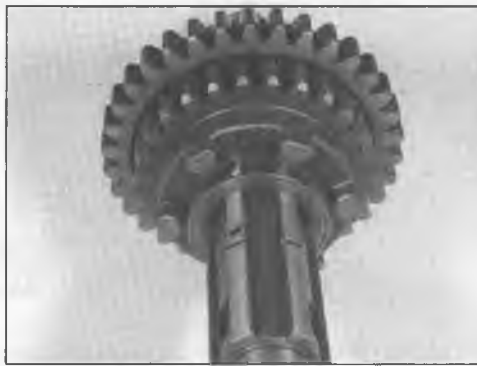
30.18a Remove the toothed washer ...
