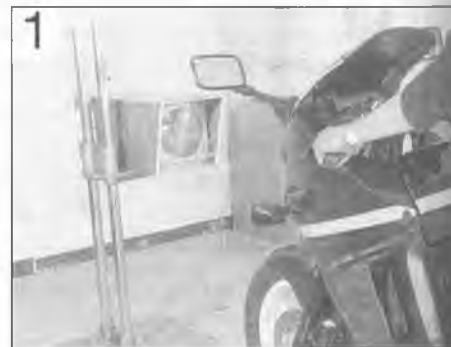
Headlight beam height checking equipment
