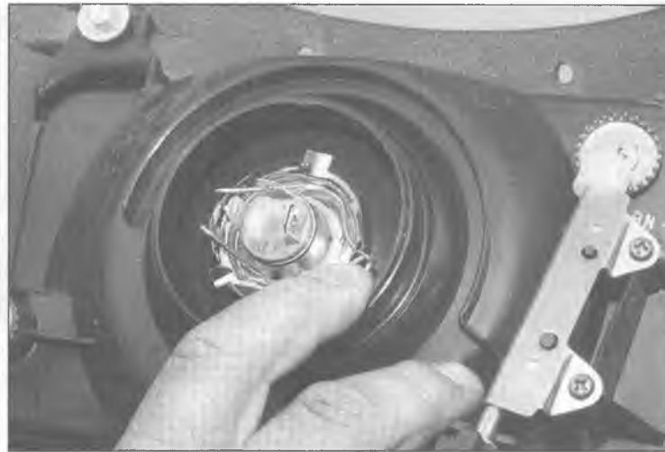
8.3a To unlock the bulb holder, release the wire retainer . . .
