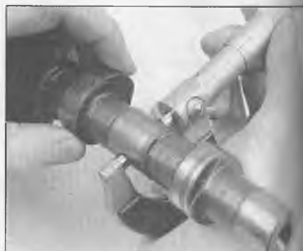
9.13b Measure the cam bearing journal with a micrometer
