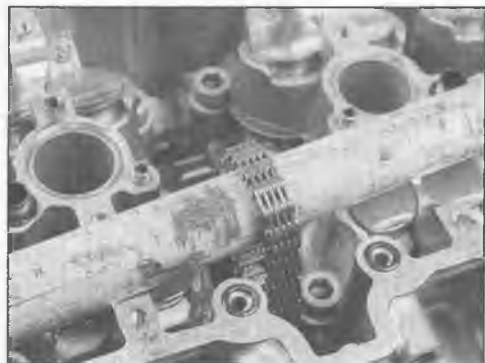
9.7 A broom handle makes a good hanger for the cam chain so the chain won't fall down into the tunnel
