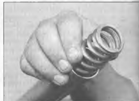
25.16e Pull out the spring; the slight taper at the lower end of the spring must face down when installed
