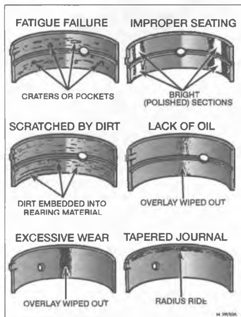
5.17 Typical bearing failures
