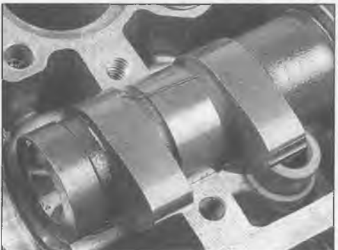
9.11 Lay a strip of Plastigauge across each bearing journal, parallel with the camshaft centerline
