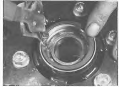
13.16 Remove the snap-ring after the grease seal has been removed
