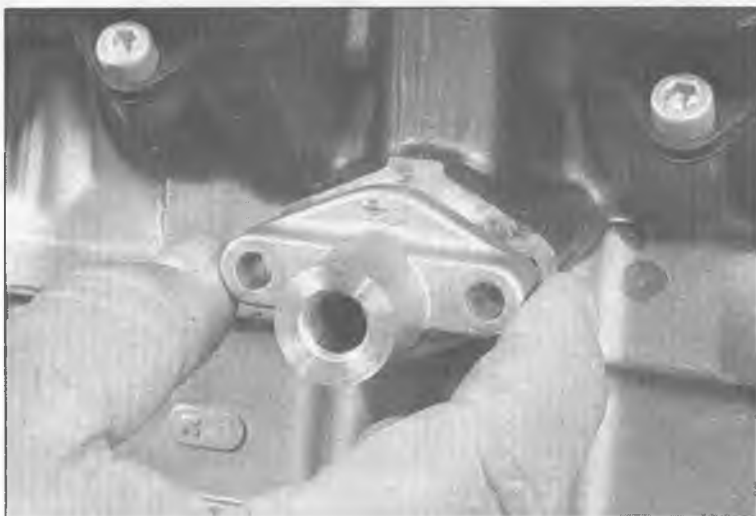
8.9 Install the cam chain tensioner with the arrow on top
