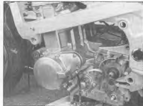
5.19 Lower the engine from the frame until the floor jack is fully collapsed
