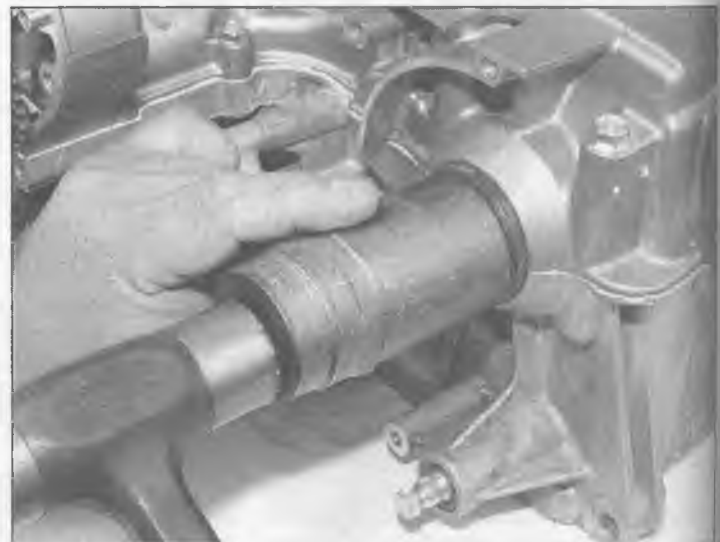
22.17 Install the seal with a socket with an outer diameter slightly smaller than the diameter of the seal
