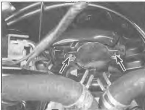
20.7 To detach the ignition main (key) switch, drill out these two shear-head bolts (arrows)
