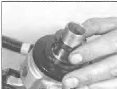
5.8 Lift the lockwasher off the steering stem . . .
