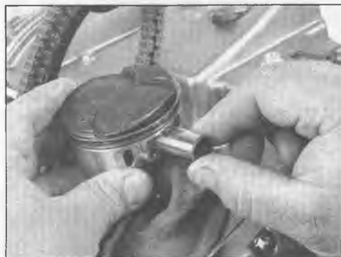
14.4a Push the piston pin through far enough to grasp it and pull it out of the piston
