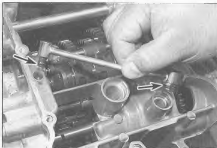
16.7c To remove the oil pipe, simply pull it straight off. Inspect the O-rings (arrowed)
