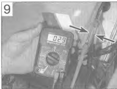
9 Continuity check of front brake light switch using a meter - note split pins used to access connector terminals
