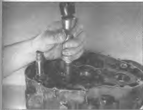
2.14 Using an impact driver to free a fastener
