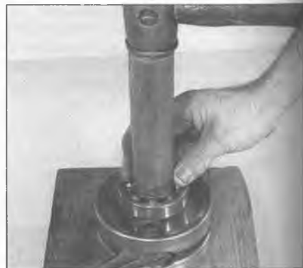
5.5 When installing a bearing on a shaft use a piece of tubing which bears only on the bearing's inner race
