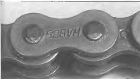
8.10 Typical chain size and type marking
