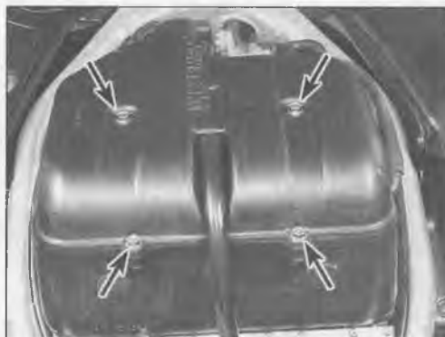
14.2b To remove the upper half of the air cleaner housing on E models, remove these bolts (arrows) . . .
