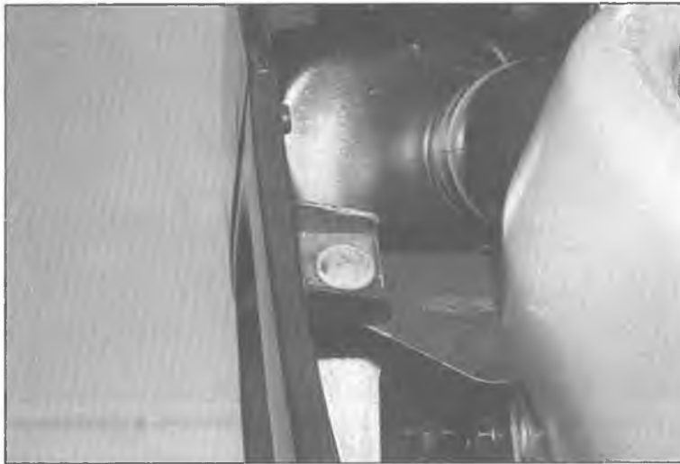
3.2 To detach the trailing edge of the middle fairing panel, remove this screw
