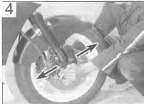
Checking the steering head bearings for freeplay
