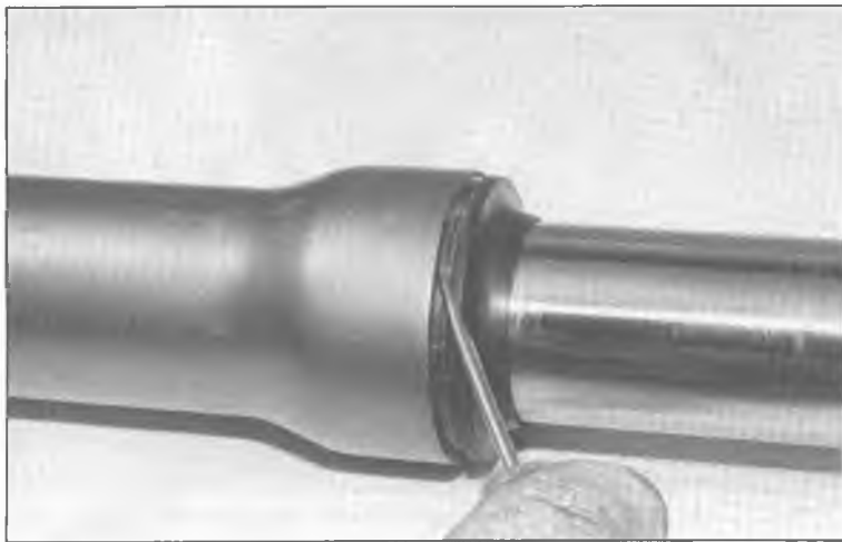
4.6 Pry the dust seal from the outer fork tube with a small screwdriver and slide it up the tube
