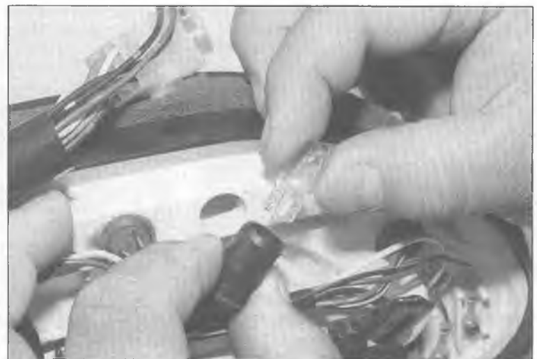
18.2b To remove a bulb from a holder, simply pull the bulb straight out
