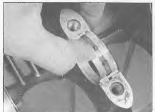
25.2 To remove a main bearing insert, push it sideways and lift it out
