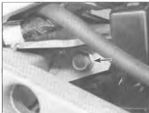
6.3 Hold the upper shock mounting bolt (arrow), then loosen the nut on the other side
