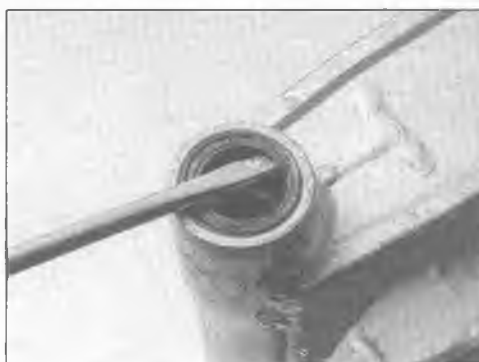
10.3b Pry out the seals with a screwdriver
