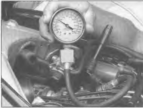
21.2 Using a compression gauge with a threaded fitting for the spark plug hole
