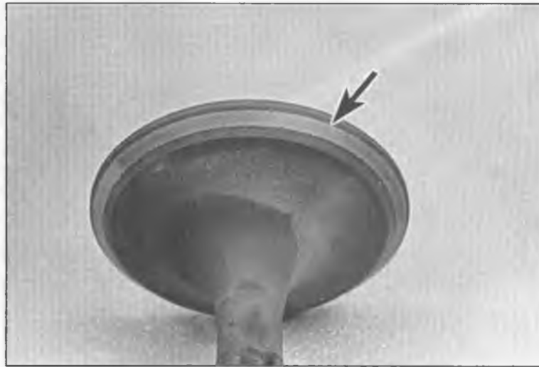
12.24a After lapping, the valve face should exhibit a uniform, unbroken contact pattern (arrowed) . . .
