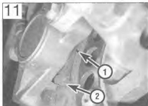
11 Brake pad wear can usually be viewed without removing the caliper. Most pads have wear indicator grooves (1) and some also have indicator tangs (2)
