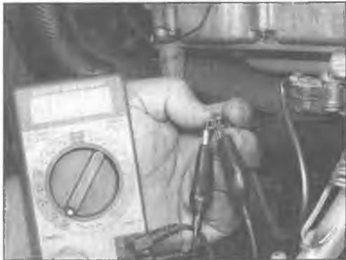
24.3 Unplug the connector, and hook up an ohmmeter to the terminals on the switch side
