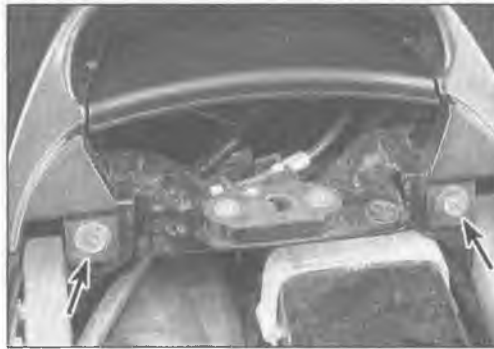
8.2 To remove the grab rail, remove these two bolts (arrows) (E model shown, D models similar)
