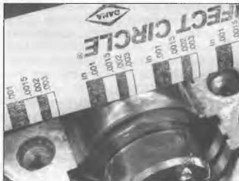
25.10 Measure the width of the crushed Plastigauge
