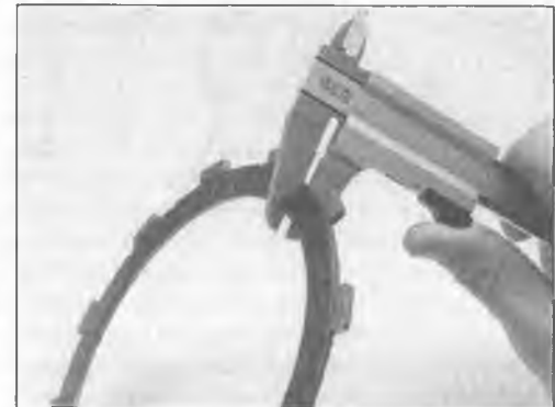
20.11 Measure the thickness of the friction plates
