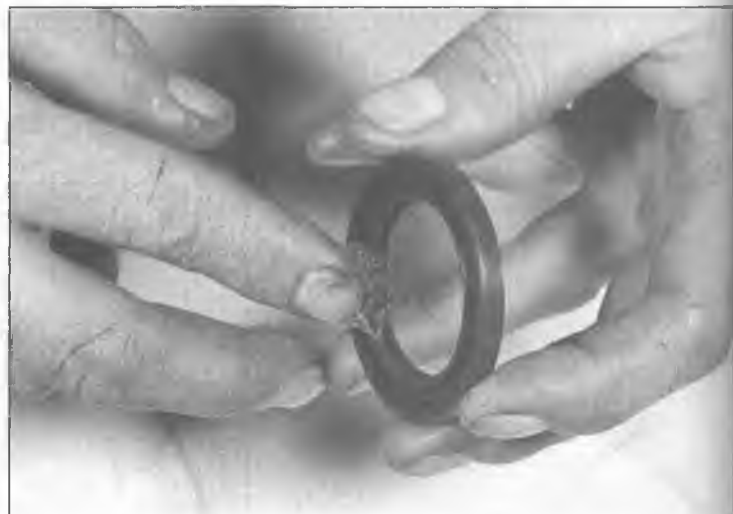
13.11 Apply a coat of grease to the lip of the seal
