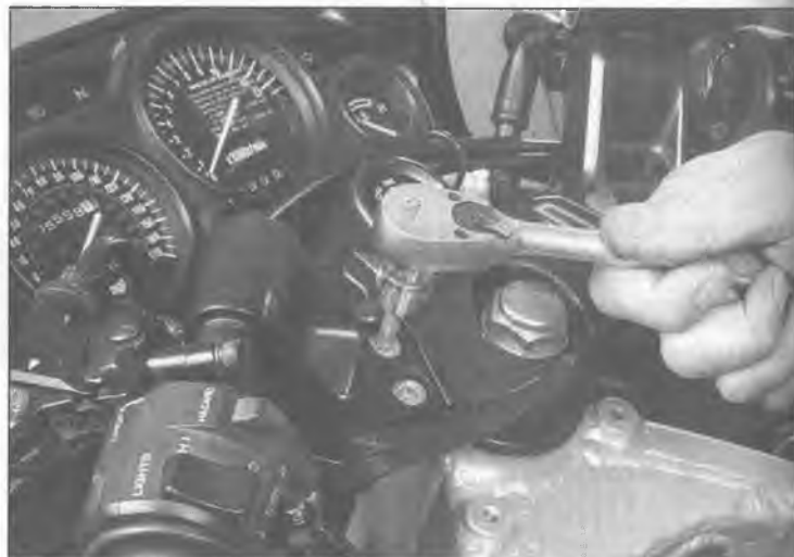
2.1b You'll need an Allen bit to remove the handlebar bolts
