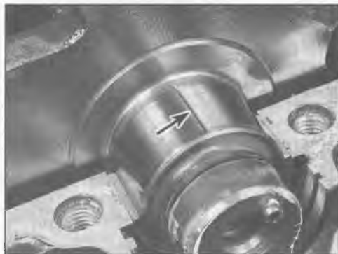
25.8 Lay the Plastigauge strips (arrowed) on the journals, parallel to the crankshaft centerline
