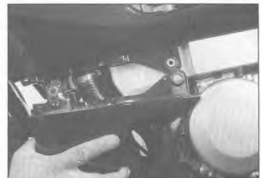
2.13 Carefully maneuver the lower fairing assembly off the bike
