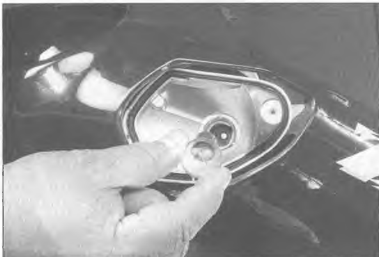
11.2b To remove a rear turn signal bulb from a holder, push it in, turn it counterclockwise and pull it out
