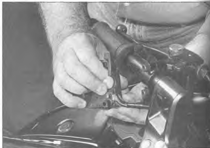
11.5 Make sure everything is installed in the switch housing before installing the housing halves
