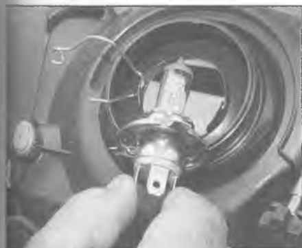
8.3b . . . then remove the bulb holder from its socket
