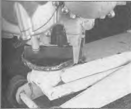
5.16 Support the engine with a floor jack
