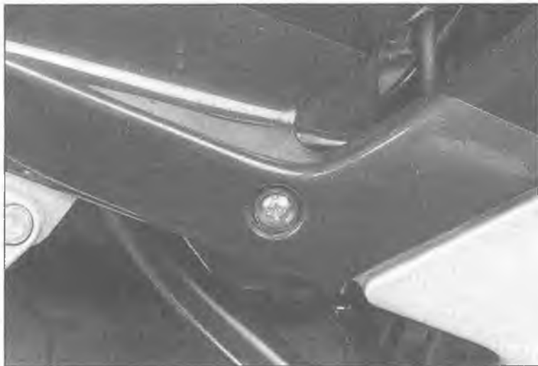
8.3b ... this screw on the side of the cover ...
