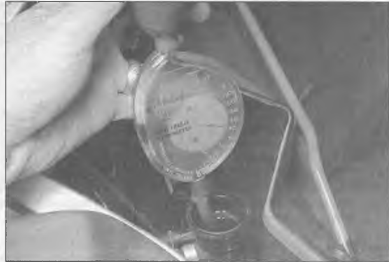
23.7 An antifreeze hydrometer is helpful for determining the condition of the coolant
