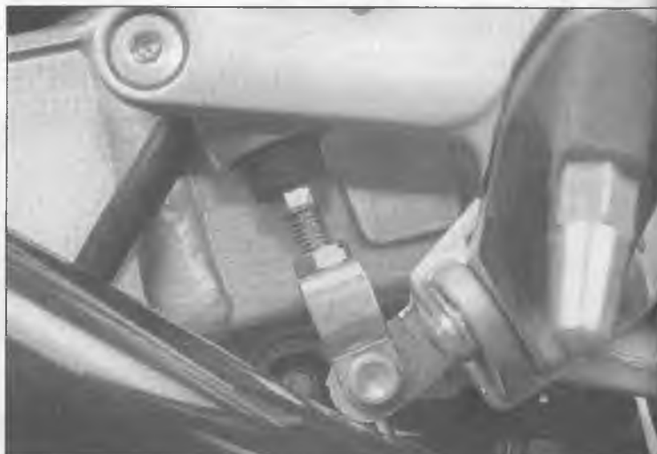
10.9 To adjust the pedal, loosen the locknut on the clevis, then screw the pushrod in or out
