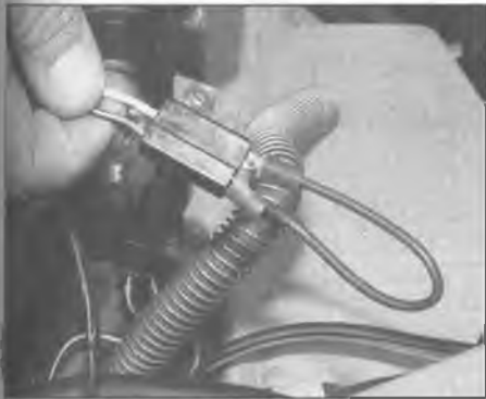
16.2 Bridge the two terminals of the female side of the connector for the fuel level sensor
