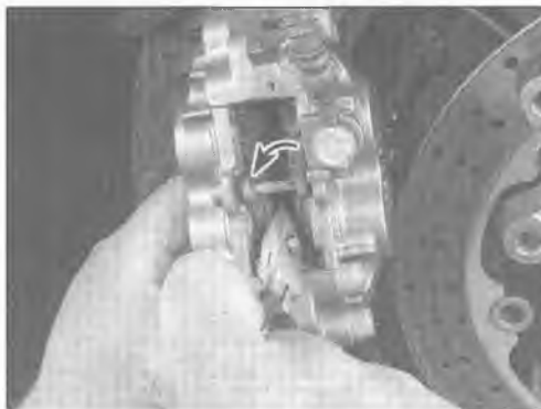
3.3b ... insert pliers between the pads and twist the pliers to depress the pistons into their bores ...
