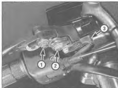
5.5 Remove the pivot nut (1) and pull out the bolt
