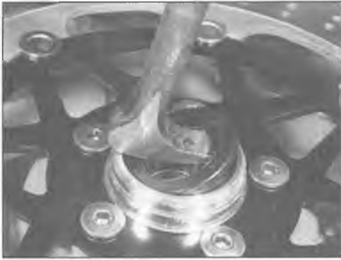
13.4b A screwdriver can be used to pry out the seal if you don't have a removal tool like this one
