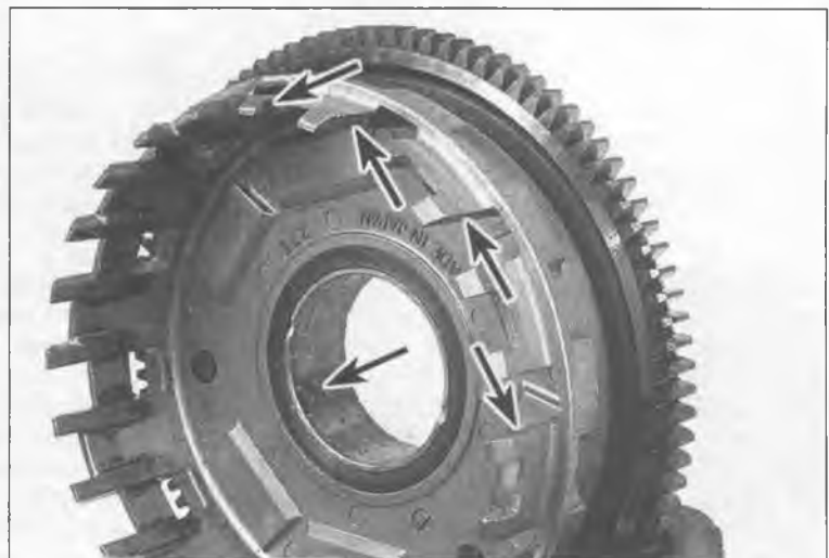
20.14 Inspect the edges of the slots and the bushing surface for heavy wear (arrowed)
