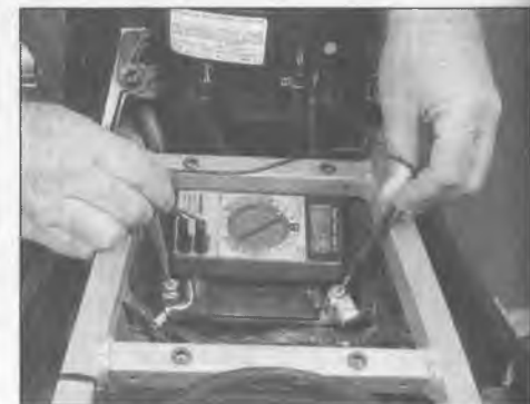
17.11 Use a digital voltmeter to measure battery voltage; it should be at least 12.6 volts
