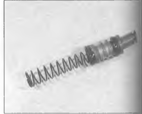
5.12 Make sure the lips of the cups face in the proper direction
