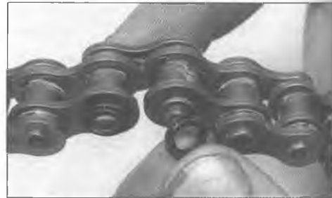
8.5 . . . install the O-rings over the pin ends . . .
