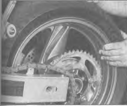
12.7 Remove the wheel, allowing the chain to rest on the swingarm
