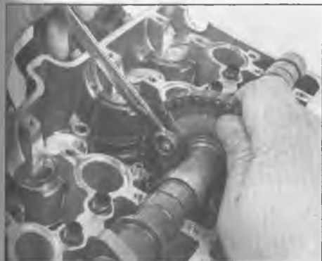
9.6d Lift the chain off the cam sprocket and rotate the cam slightly to get at the other bolt
