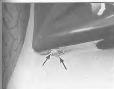
2.11 To detach the forward ends of the lower fairing halves, remove these two bolts (arrows)
