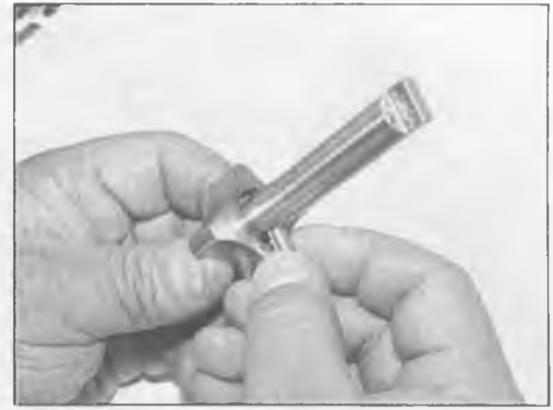
17.14b Don't lose this pin that locks the inner rotors to the shaft
