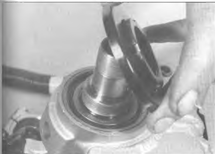
5.9b ... and lift off the nut and bearing cover
