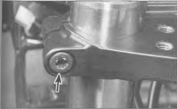
3.7a To detach the fork tube from the bike, remove the upper triple clamp bolt (arrow) . . .
