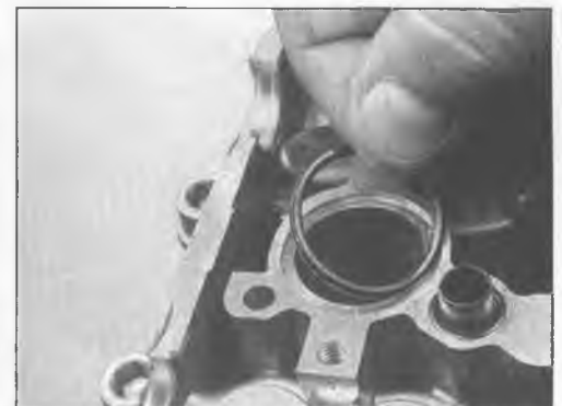
9.6f Remove all four spark plug hole O-rings and discard them; don't lose the four dowels
