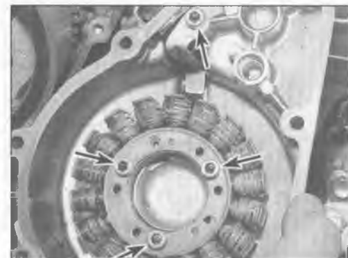
32.3 Remove the Allen bolts (arrows), the clamp retaining bolt (arrow) and the harness clamp
