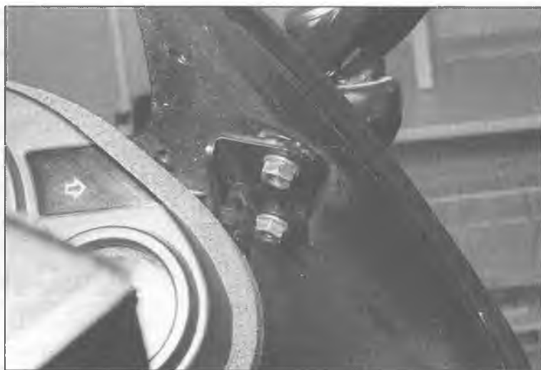
5.1 To detach either mirror from the upper fairing, remove these two nuts (arrows) (E model shown)
