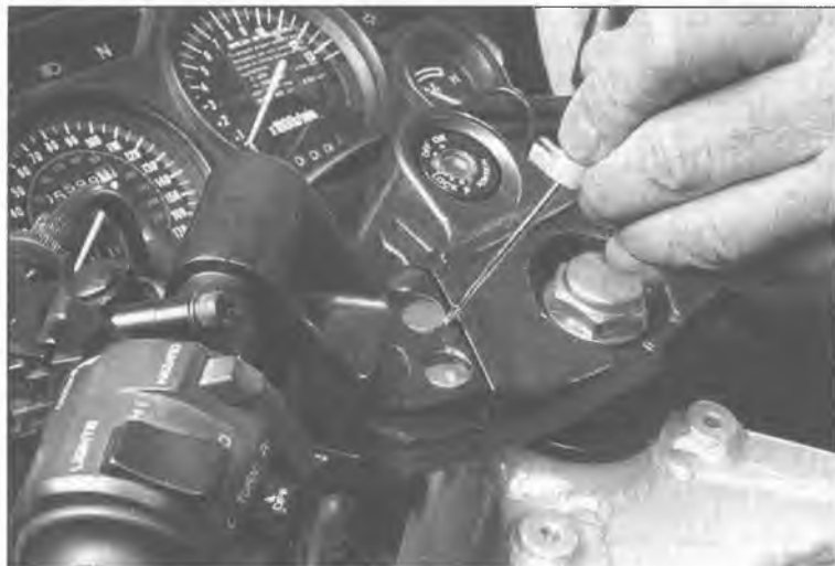
2.1a To get to the handlebar bolts, pry out these two caps with a small screwdriver
