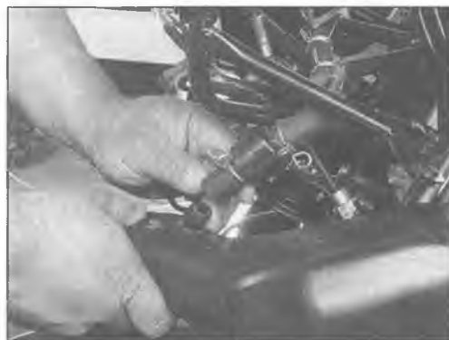
6.16 Loosen this hose clamp, slide it back and detach the hose from the ram air duct
