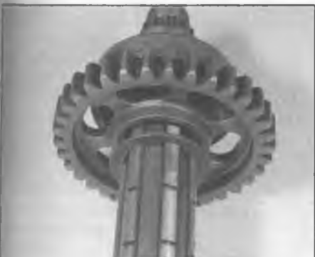
30.19b ... the toothed washer and second gear ...
