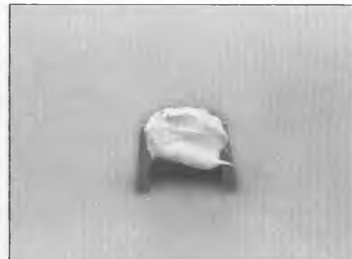
12.27 A dab of grease will hold the keepers/collets in place while the spring compressor is released
