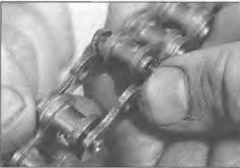
8.3 . . . and separate the chain link
