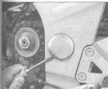
9.4 Pry off this protective cap on the left side of the bike and loosen the nut underneath
