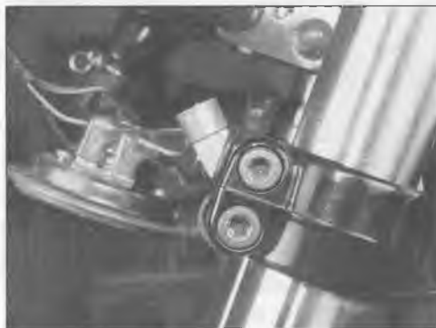
15.7b . . . and loosen the fork lower pinch bolts (fairing removed for clarity)
