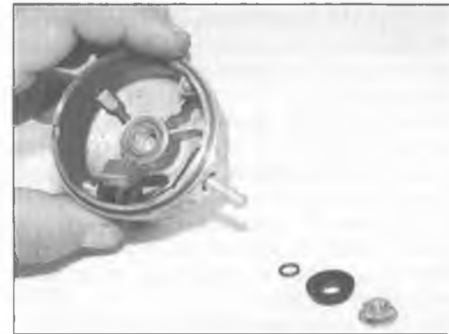
28.12b Install the O-ring first, then the insulator, then the nut
