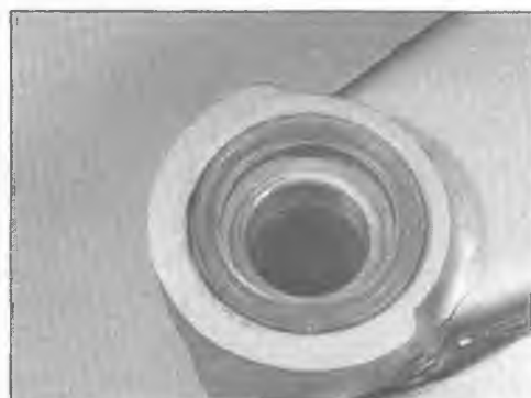
10.6 Make sure the seal faces are flush with the pivot boss of the swingarm
