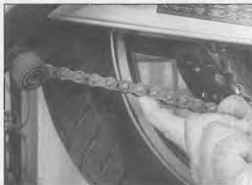
2.3 Push up on the bottom run of the chain and measure the slack midway between the two sprockets
