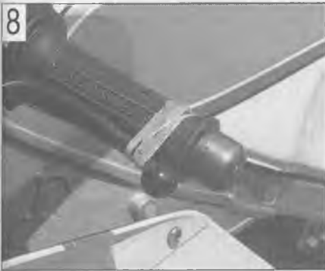
Hold clutch lever back against the handlebar with elastic bands or a cable tie
