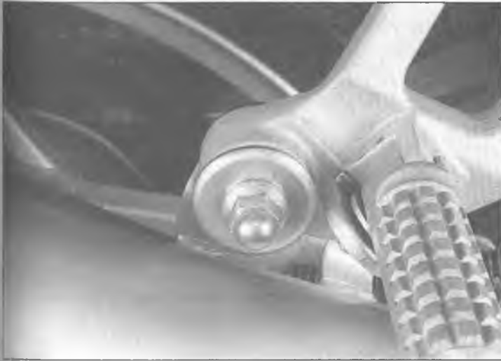
13.4 To detach a muffler, remove this bolt, washer and nut
