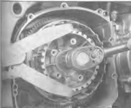
20.7a Hold the clutch hub with a clutch holder tool and break the clutch hub nut loose
