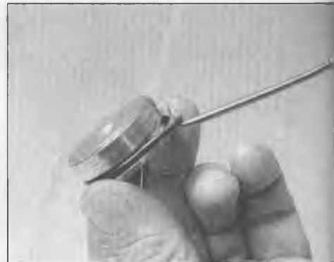
25.16b Inspect the top plug O-ring - if it's damaged, discard it and get a new one
