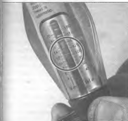
4.1 Set the torque wrench index mark to the setting required, in this case 12 Nm
