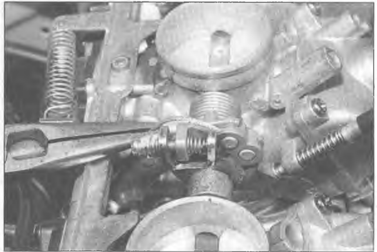
5.7a Lift the carburetor assembly, flip it over, pull the cable toward the pulley to create some slack . . .
