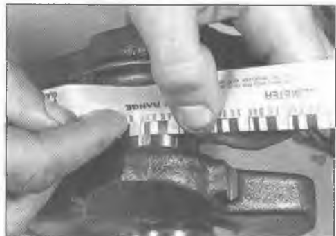
3.16 Measuring the width of the crushed Plastigauge
