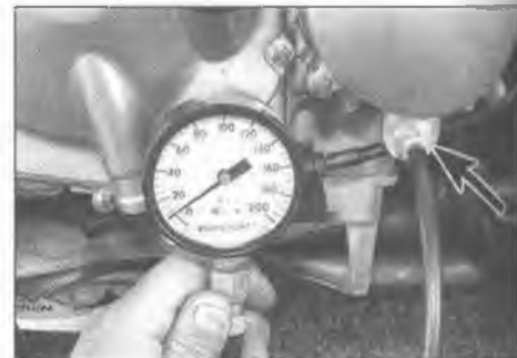
3.21 Oil pressure gauge and take-off point adapter (arrow)
