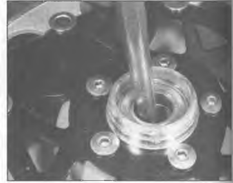
13.5 Once the snap-rings have been removed, drive the bearings from the hub with a brass drift
