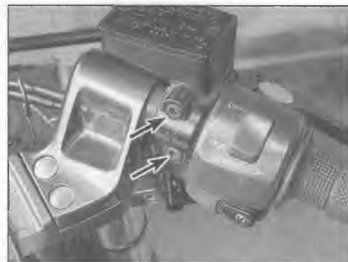
5.6 To detach the master cylinder from the handlebar, remove these two Allen bolts (arrows)
