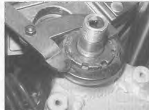
15.8 Tightening the steering stem locknut with the Kawasaki tool (upper triple clamp removed for clarity)
