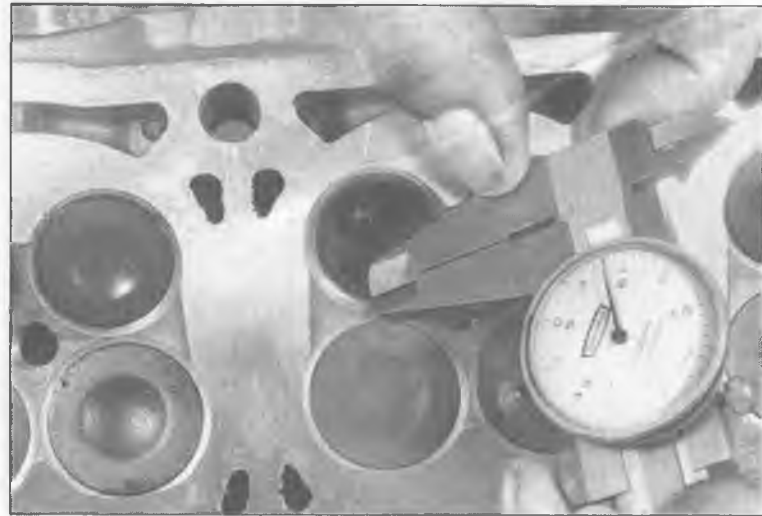
12.15 Measuring valve seat width
