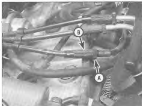
11.2a Loosen the locknut (A), and back off the adjuster nut (B) to put some slack in the choke cable
