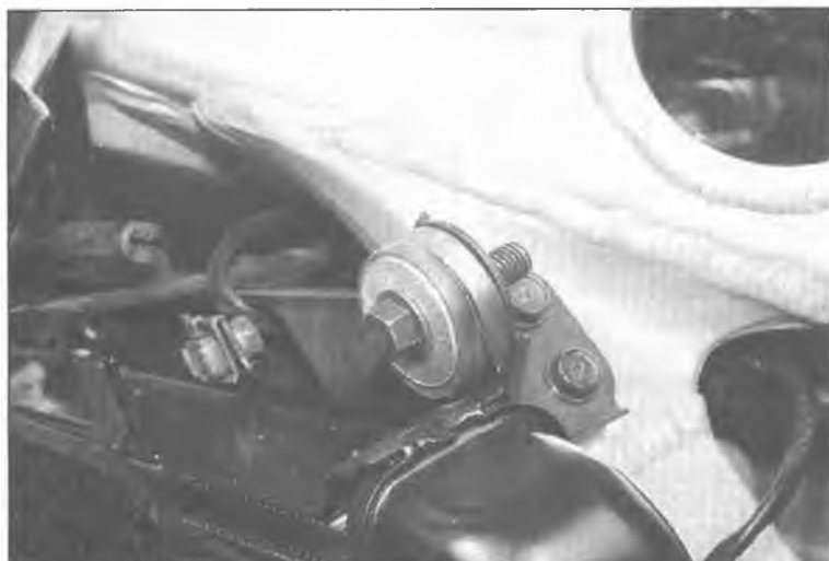
8.6 Remove the bolts that attach the upper corners of the radiator to their frame brackets
