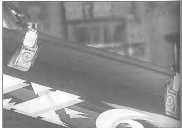
8.3c ... these two screws (don't lose the cargo hooks!) ...
