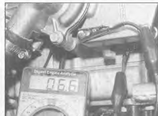
23.3b Unplug the light green wire from the switch and attach an ohmmeter to the switch and to ground
