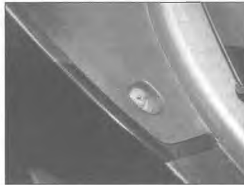
4.2a To detach the instrument cluster trim panel from the fairing on a D model, remove this screw . . .
