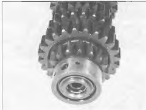
30.2a Slide off the needle bearing outer race . . .
