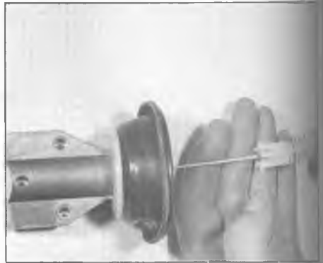
7.4a Separate the jet needle from the throttle piston
