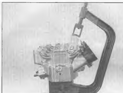
12.7a Compress the valve spring with a valve spring compressor . . .
