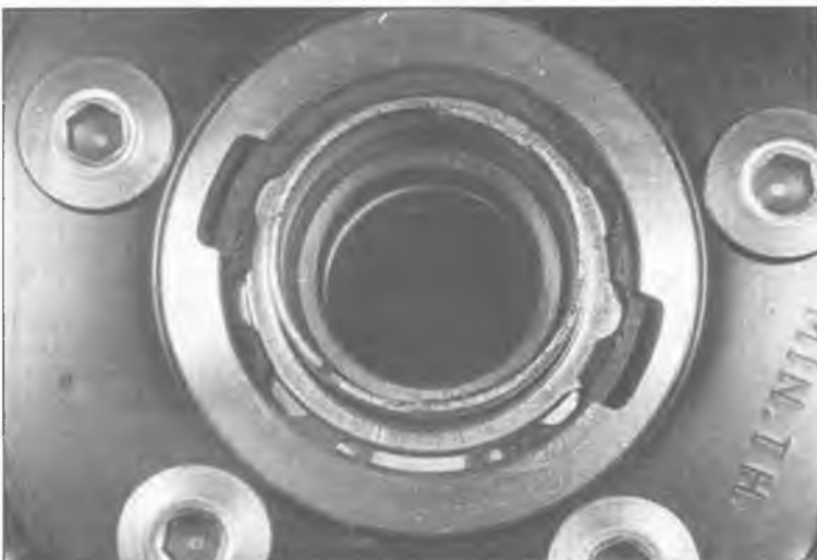
13.10 Install the speedometer drive and secure it with the snap-ring
