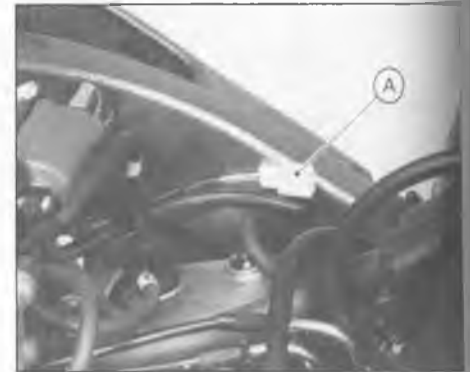
17.6 Unplug the two-pin electrical connector (A) for the low fuel level sensor (D models)
