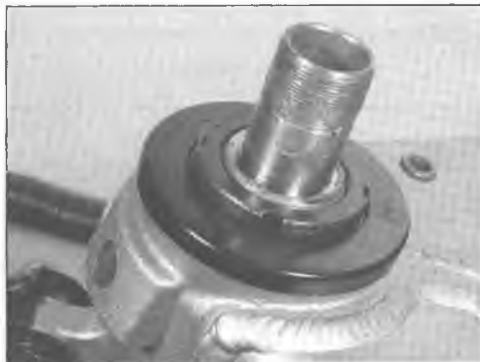
5.22b Install the bearing cover and tighten the adjuster nut until all play has been removed
