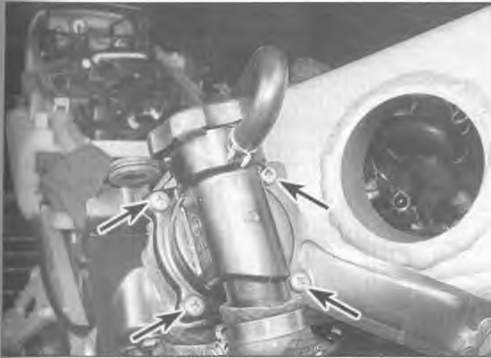
6.4 Remove the four screws (arrows) that attach the cover to the thermostat housing
