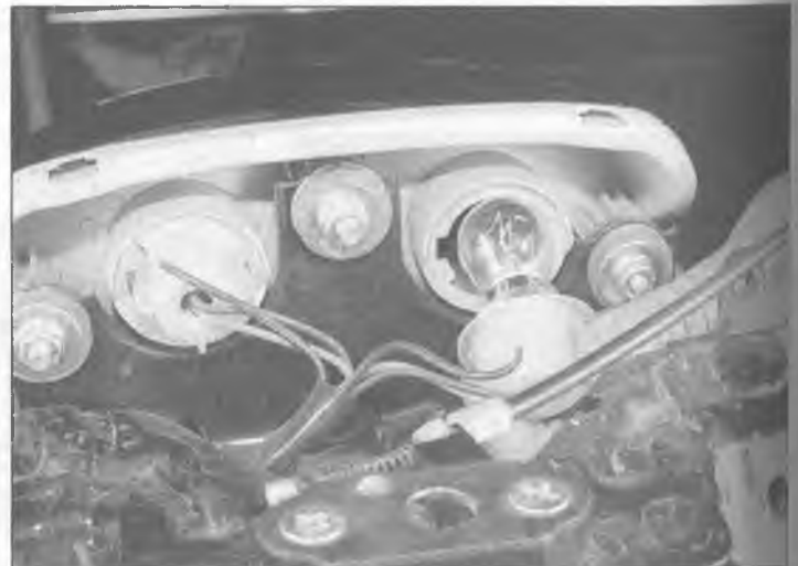
11.5 To replace a tail light/brake light bulb, push in and turn counterclockwise, then pull out
