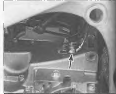
5.14 Remove this bolt (arrowed) from the top of the case and detach the ground strap
