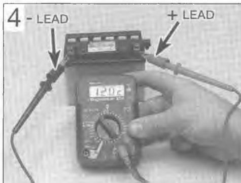
Measuring open-circuit battery voltage
