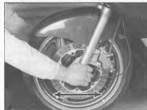
15.4 Try to move the forks back-and-forth; if you feel any play, adjust the steering head bearings
