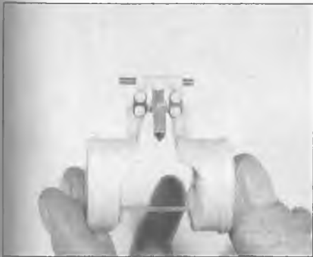
7.6c ... and lift out the float, together with the needle valve
