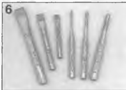
4 Vernier gauge 5 Circlip pliers (internal and external, or combination) 6 Set of cold chisels and punches
