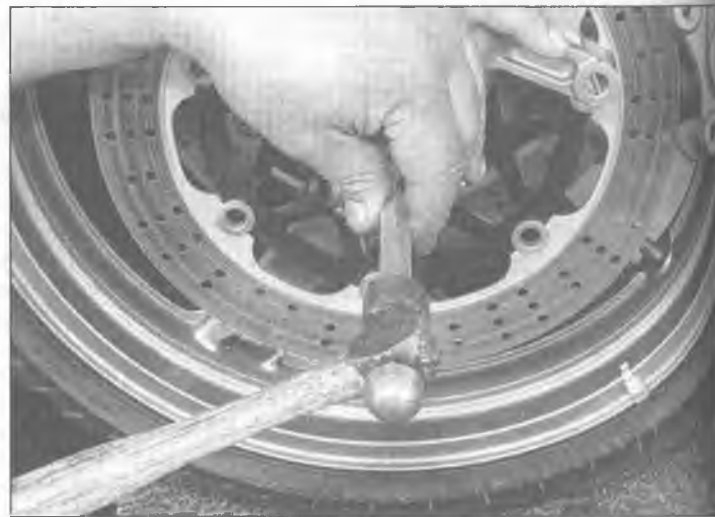
11.5b If the axle is difficult to remove, drive it out from the left side with a hammer and punch
