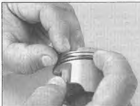
15.9b Do NOT use a ring installation tool to install the oil ring side rails
