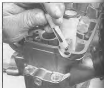
12.7b . . . and remove the collets (keepers)
