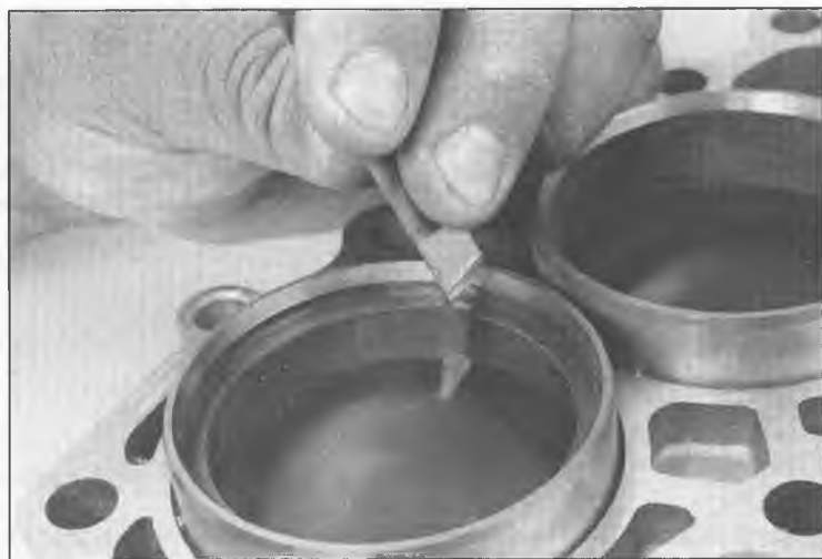
15.3 Measure the piston ring end gap with a feeler gauge
