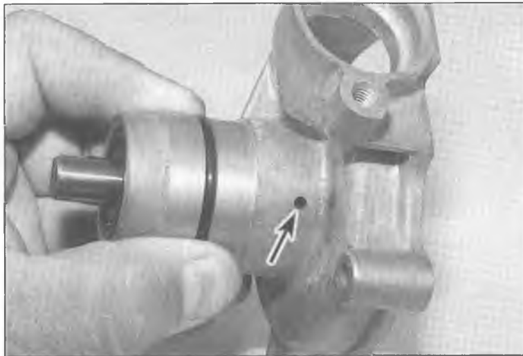
9.14 Inspect the "weep hole" carefully
