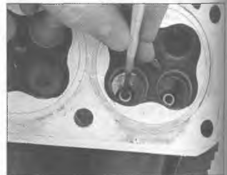
3.9 Expand the small hole gauge in the bore, lock its position ...
