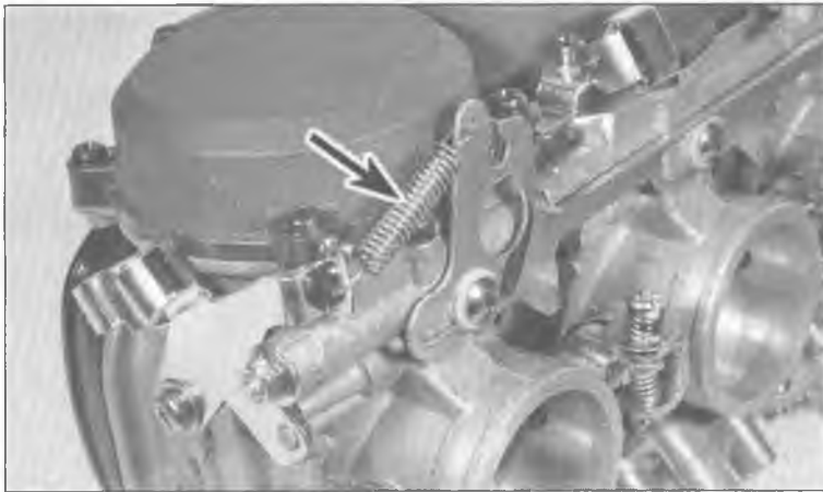
7.2a Remove the choke shaft spring (arrow) . . .
