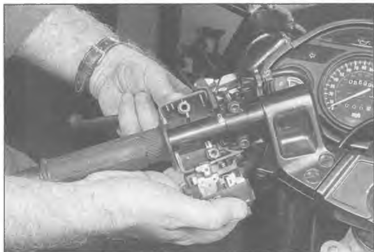
11.3b . . . separate the housing halves and disengage the cable from the lever
