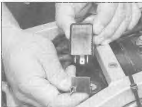
13.8 Lift up the relay to free it from its rubber mounting, then unplug it from the base (E model shown)
