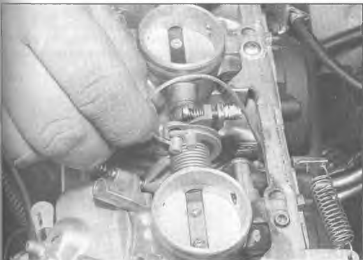
5.7b . . . disengage the throttle cables from the throttle pulley . . .
