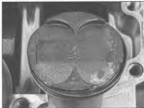
14.3a Scribe or mark the number of each piston into the piston crown
