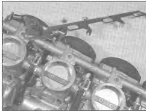
7.2d . . . separate the choke shaft from the carburetors
