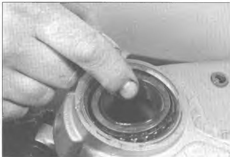
5.11 Lift the upper steering head bearing out of the steering head
