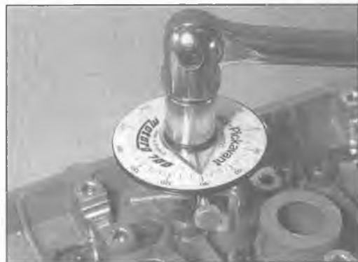
Angle-tightening cylinder head bolts
