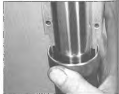
4.15f Tap the seal into place until it seats in the outer fork tube (half of the driver removed for clarity)
