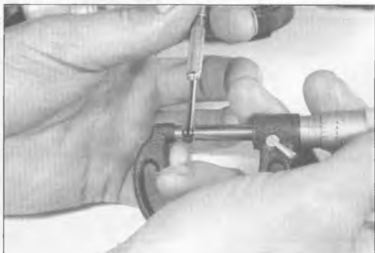
12.16b . . . then measure the gauge with a micrometer
