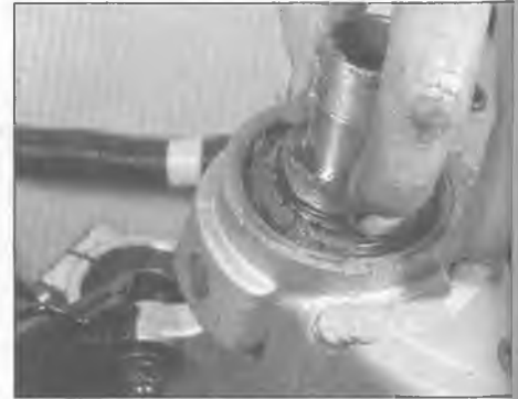
5.22a Install the upper bearing and the O-ring
