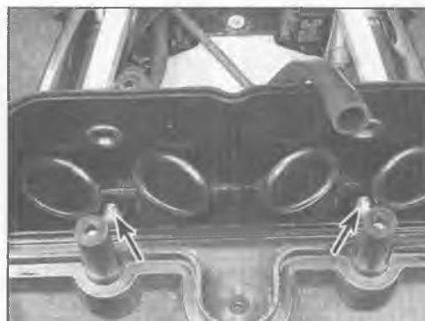
4.5b . . . remove the rear mounting bolts (arrows) . . .
