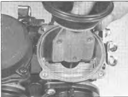
7.3e Lift the throttle piston out
