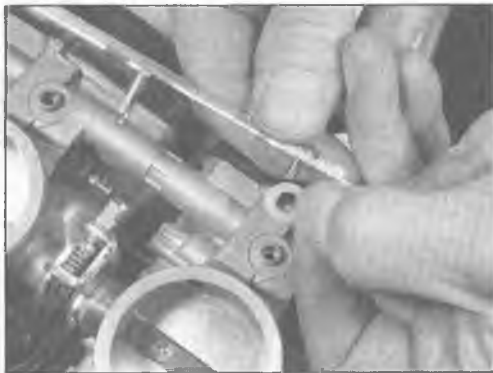
7.2c . . . there are two plastic washers for each screw, one on each side of the choke shaft . . .
