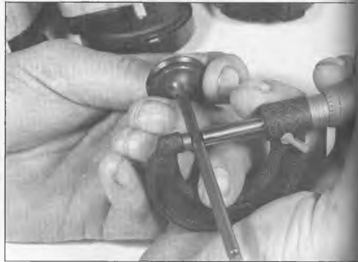
12.18a Measuring valve stem diameter
