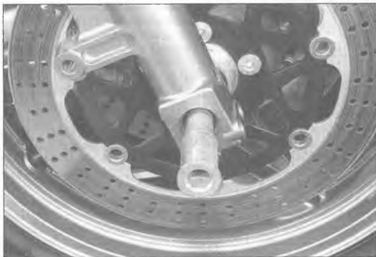
11.5a Pull out the axle from the right side
