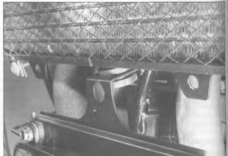
8.7 Lift the radiator to disengage the pin on its lower edge from the grommet on top of the oil cooler
