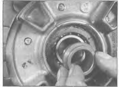
13.17 Lift out the coupling collar
