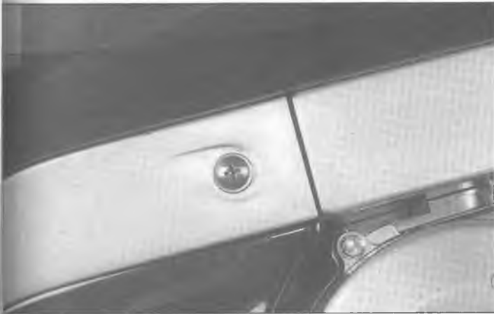
2.7 Remove the cover screws from each side of the bike (E model shown)
