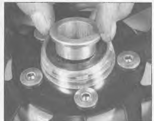
13.4a Lift the spacer out of the wheel
