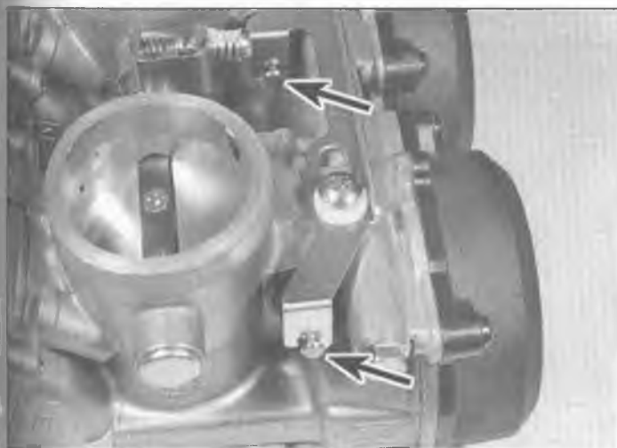
8.14a Make sure the choke shaft engages all four plungers (arrows)
