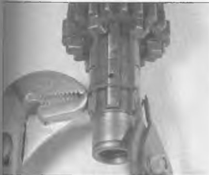
30.5b ... holding the back of the snap-ring with pliers to prevent it from twisting
