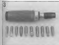
1 Torque wrench (small and mid-ranges) 2 Conventional, plastic or soft-faced hammers 3 Impact driver set
