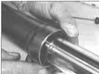
4.15g Compress the retaining ring and fit it securely into its groove
