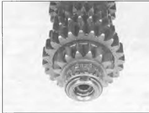
30.2b . . . then remove the snap-ring and bearing
