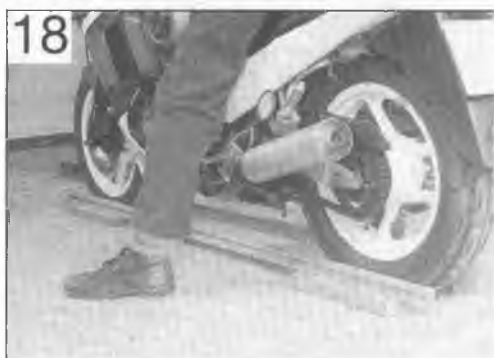
18 Two straightedges are used to check wheel alignment
