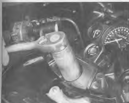
15.7a Loosen the steering head nut . . .
