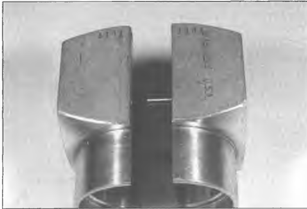
4.15b Using a split-type seal driver (this is a Kent-Moore, but any suitable equivalent will work) . . .
