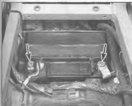
17.12 Remove the cables from the terminals (remove the negative cable first) and pull the battery straight up
