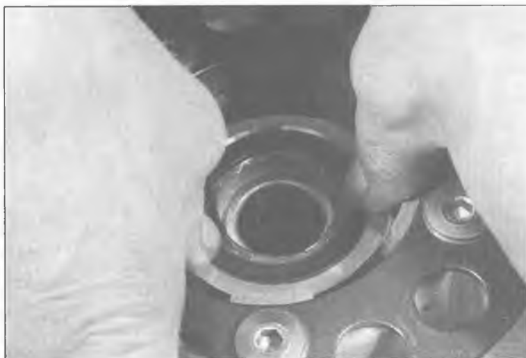
13.33 Press the seal into the hub with your thumbs
