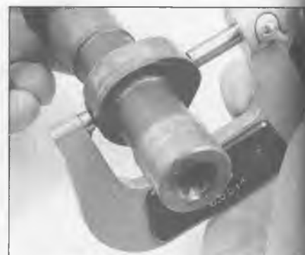
9.9b Measure the height of the camshaft lobes with a micrometer
