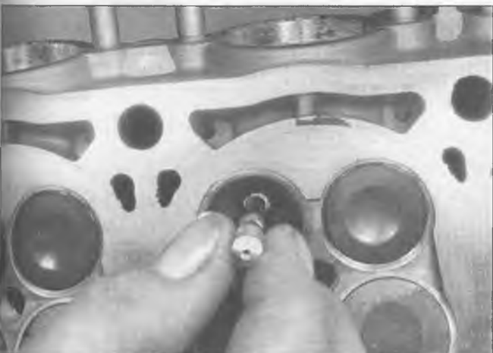
12.16a Measure the valve guide inside diameter with a hole gauge . . .
