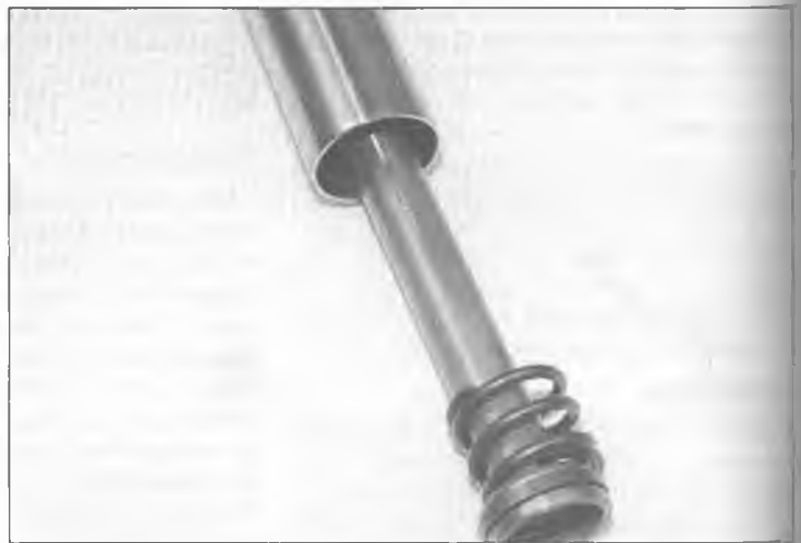
4.9 Invert the inner fork tube and remove the piston cylinder unit and spring
