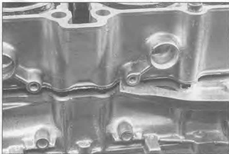
13.3a Pry between a mounting bolt boss on the crankcase and a boss for the lower water pipe
