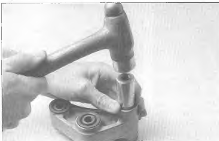
7.10 Drive in the new needle bearings with a socket that just fits into the bore of the rocker arm
