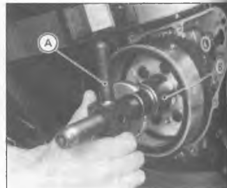
32.5 You'll need a rotor puller (A) and flywheel puller (B) to remove the alternator rotor
