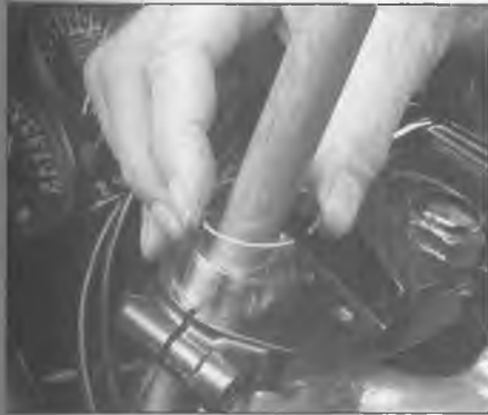
25.24a Depress the plug with a large punch or Phillips screwdriver, remove the wire retaining ring . . .
