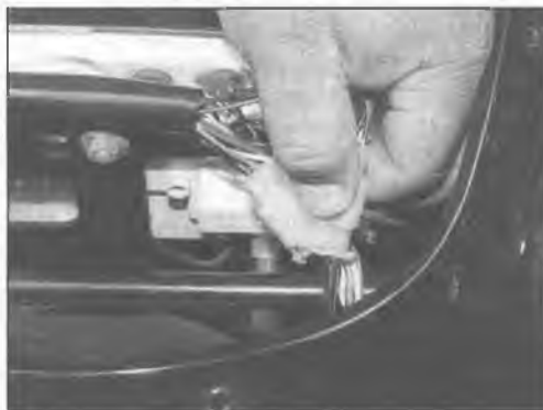
15.2a Unplug the electrical connector for the instrument cluster
