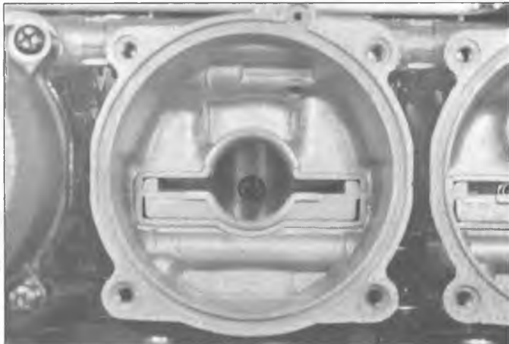
7.18 Check the piston insert and the needle jet for wear or damage
