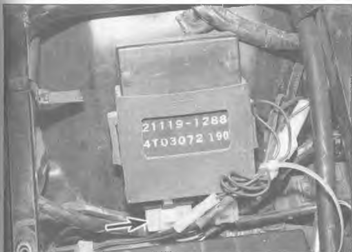
4.2a Unplug the pickup coil connector from the IC igniter (D models)
