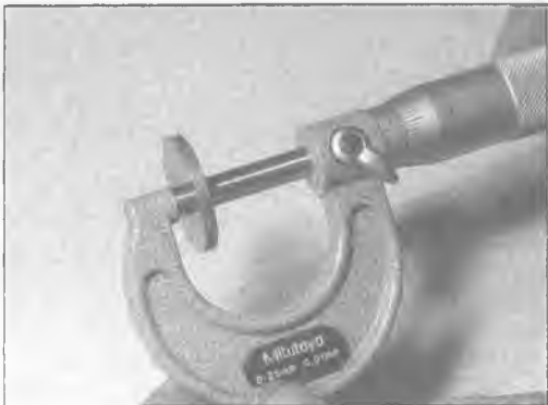
Tappet shims are measured with a micrometer
