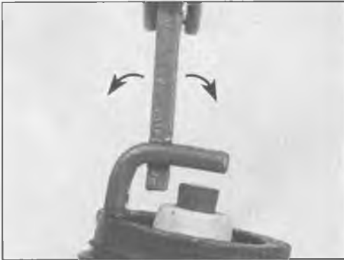
3.6b To change the gap, bend the side electrode; be careful not to crack the center electrode insulator
