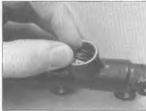
6.8b Remove the O-ring from the bore and discard it
