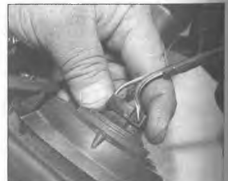
7.2 Unplug the electrical connector for the headlight
