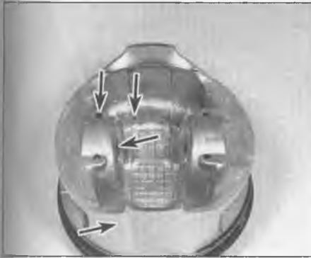
14.11 Check the piston pin bore and the skirt for wear, and make sure the oil holes are clear (arrowed)
