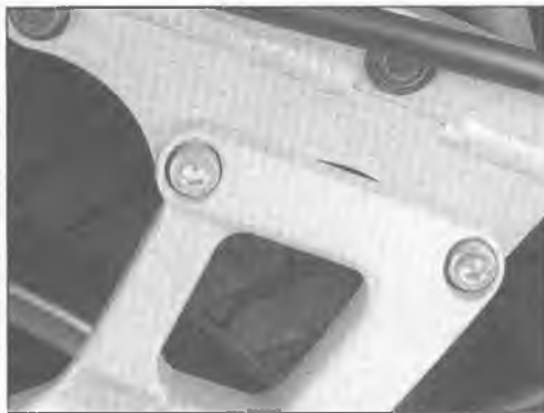
11.12 To remove either passenger footpeg bracket, remove the two Allen head bolts
