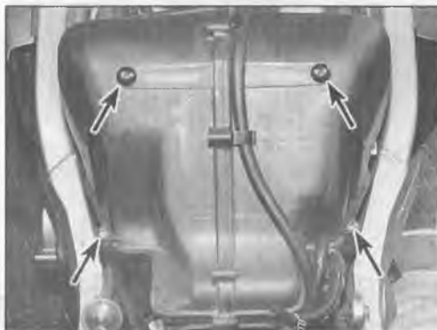
14.2a To remove the upper half of the air cleaner housing on D models, remove these screws (arrows)
