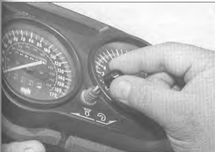
16.5a Before removing the cover from the instrument cluster, unscrew the trip reset knob
