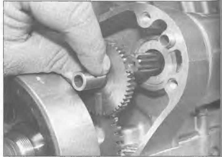
28.17 Remove the starter motor idler gear and bushing and inspect both for excessive wear
