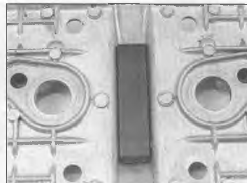
7.10 Flip the valve cover upside-down and inspect the chain rubbing block - if it's worn, replace it
