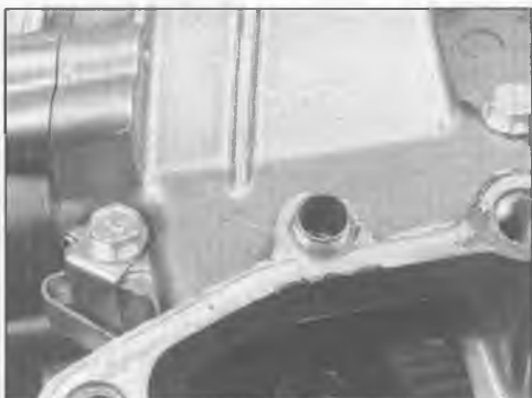
13.5 Remove the positioning dowels from the crankcase
