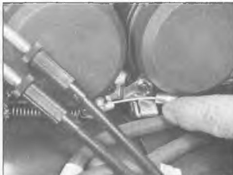
11.2b Pull the cable free of the bracket and slide the cable through the slot in the bracket
