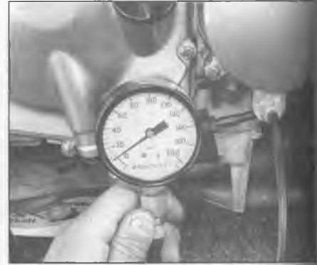
17.2 Remove the bolt from the end of the main oil passage, attach an oil gauge and start the engine
