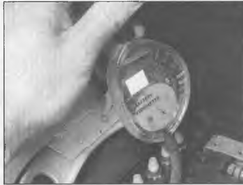
17.5 On D models, check the battery's specific gravity with a hydrometer
