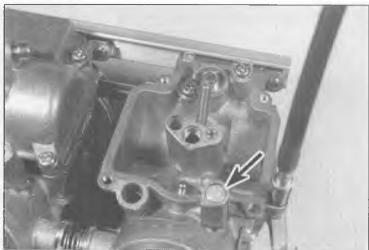
7.10a The pilot screw on US models is beneath a plug (arrow)
