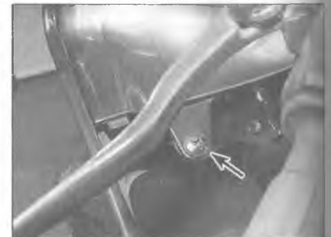
4.2e To detach the instrument cluster trim panel from the fairing on an E model, remove the screws (arrow, and below the right end of the panel)
