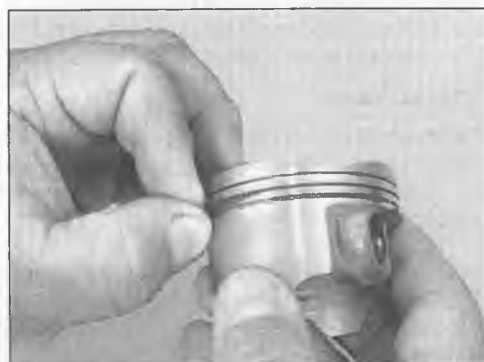
15.9a When installing the oil ring expander, make sure the ends don't overlap
