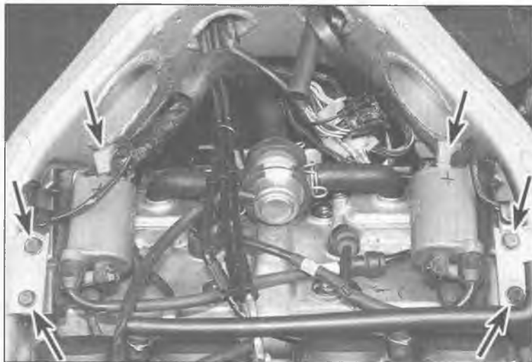
3.10b Remove the mounting bolts (arrows), and label and unplug the leads (arrows) - E models
