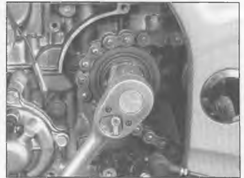
16.6b . . . and loosen the sprocket nut with the transmission in first gear and someone applying firm pressure to the rear brake pedal
