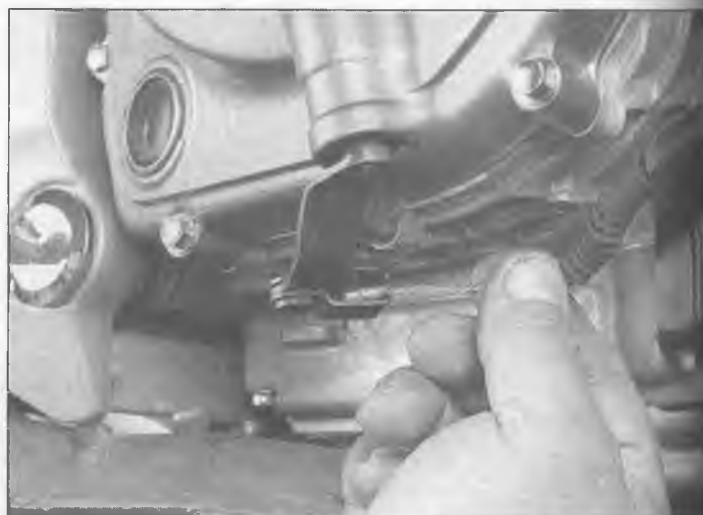
19.7 To disconnect the cable from the lever, push the lever forward and disengage the cable
