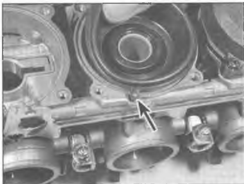
7.3d ... and separate the diaphragm from its groove and the locating tab (arrow) from its notch
