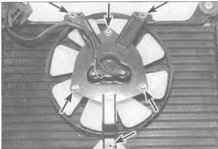
4.6 To detach the fan, remove the bolts (arrows); to separate the motor, remove the screws (arrows)
