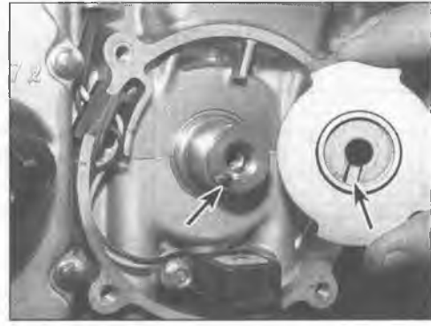
5.4 Align the notch in the timing rotor with the pin on the crankshaft (arrows)
