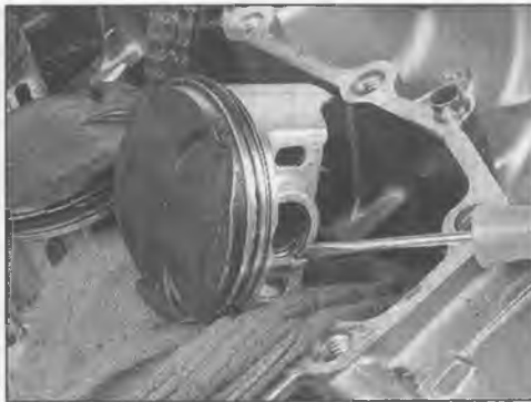
14.3b Pry the piston pin circlip loose with a small screwdriver
