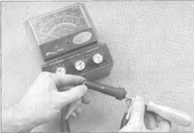
2.5 Unscrew the spark plug caps from the plug wires and measure their resistance with an ohmmeter
