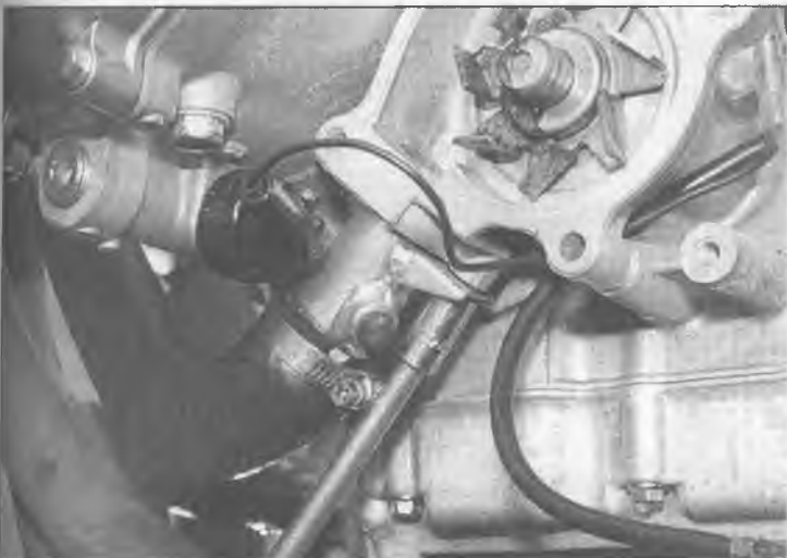
9.12 Remove the drain plug housing retaining bolt and detach the housing and outlet hose
