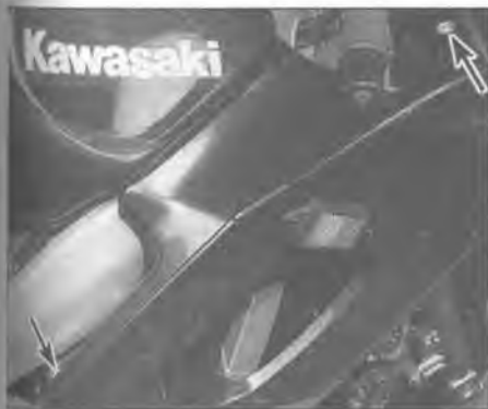
6.12b To remove the right trim panel on E models, remove these screws (arrows)
