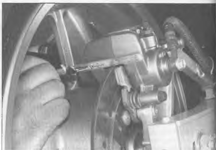
9.3 Check the rear brake pads by looking into the caliper from the rear of the machine
