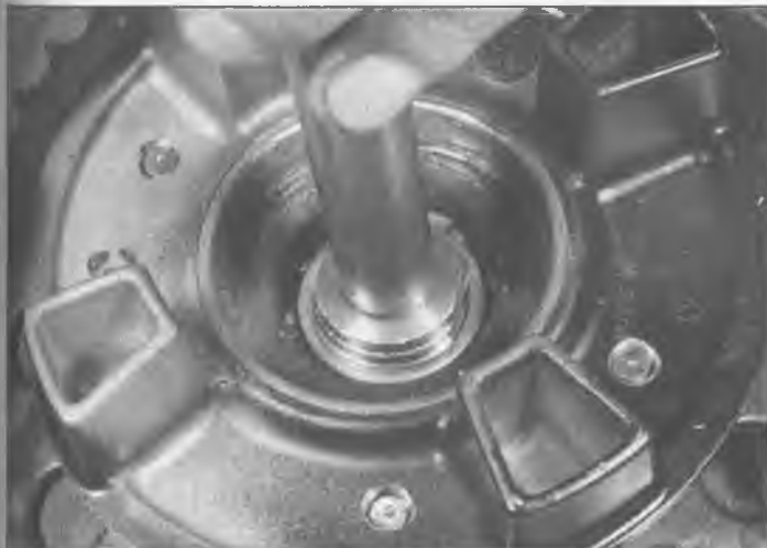
13.18 Drive out the coupling bearing
