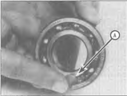
13.8 Press grease into the open side of the bearing (A) until it's full
