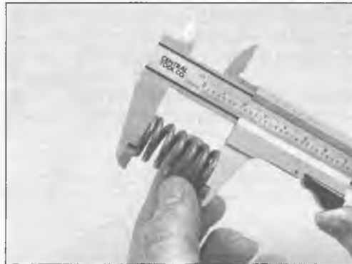
20.10 Measure the clutch spring free length
