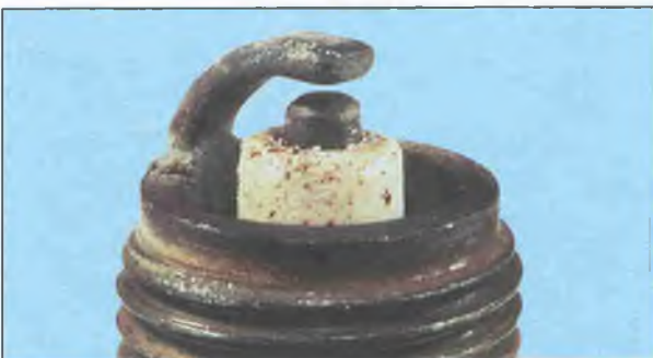
Overheating – A blistered white insulator and glazed electrodes. Caused by ignition system fault, incorrect fuel, or cooling system fault.
