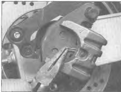
3.10a Before removing the pads from the rear caliper, remove this retaining pin clip ...
