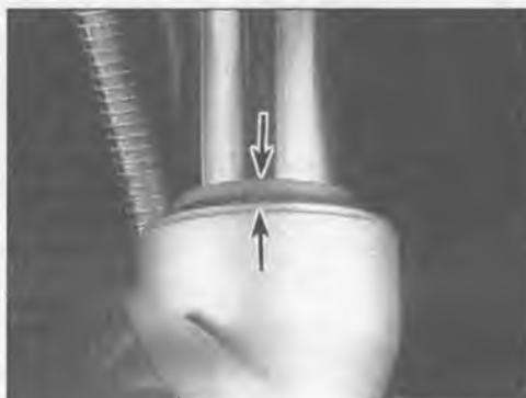
20.3 Inspect each fork seal for leaks at the indicated areas (arrows)
