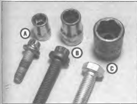
2.2 External Torx (A), splined (B) and hexagon (C) fasteners, with corresponding sockets
