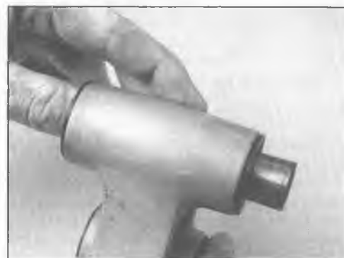
7.6b Push the sleeves out of the rocker arm (shown) and the swingarm (not shown)
