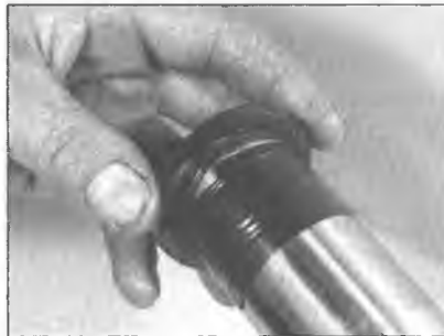
4.15e Wrap the top of the fork tube with tape to prevent the lip on the new seal from damage
