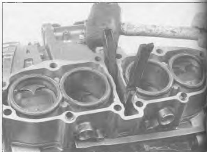
13.3b If the cylinder block is stuck, use a rubber mallet to knock it loose
