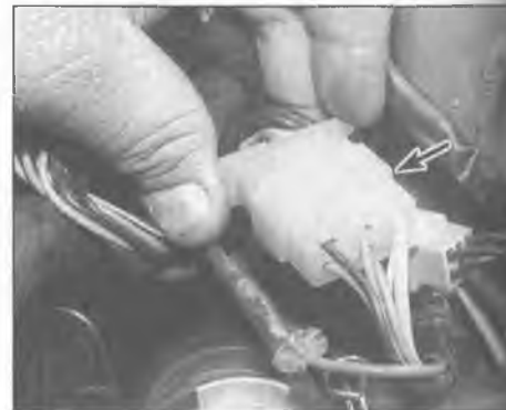
20.2 Unplug the electrical connector (arrow) for the ignition main (key) switch
