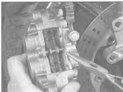
3.3a To remove the brake pads, pull out the retaining pin clip ...
