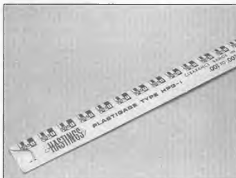
6.2b Plastigauge is needed to check the crankshaft, connecting rod and camshaft oil clearance
