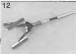
10 Piston ring removal and installation tool 11 Piston ring clamp 12 Cylinder bore hone (stone type shown)
