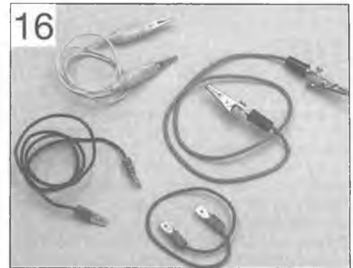
16 A selection of jumper wires for making earth (ground) checks
