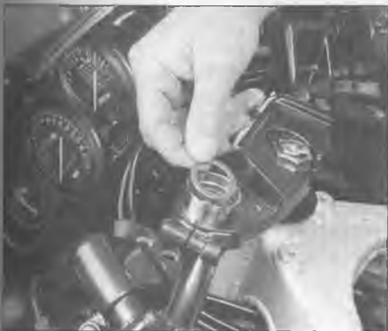
25.24d . . . and remove the spring seat (the large washer) with a magnet
