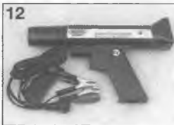
10 Wire stripper and crimper tool 11 Multimeter (measures amps, volts and ohms) 12 Stroboscope (for dynamic timing checks)
