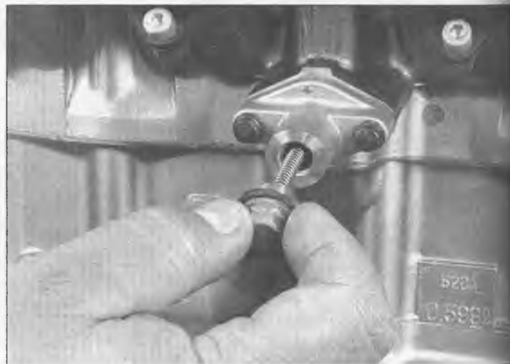
8.10 Install the spring and guide pin into the tensioner, then collapse the spring with the cap bolt
