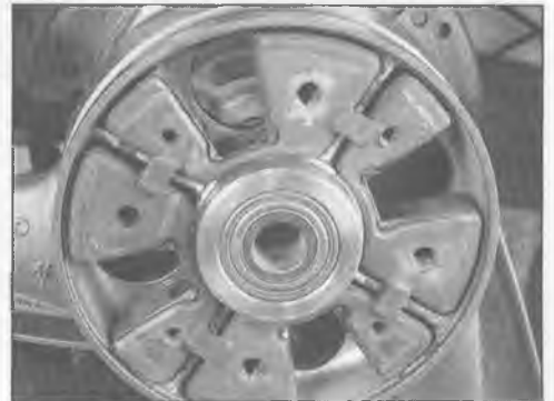
17.3 To remove the rubber coupling damper, simply pull it out of the wheel
