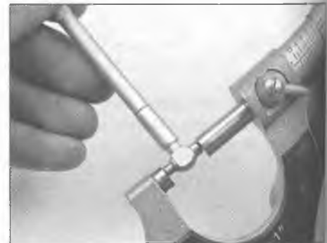
3.8 ... then measure the gauge with a micrometer
