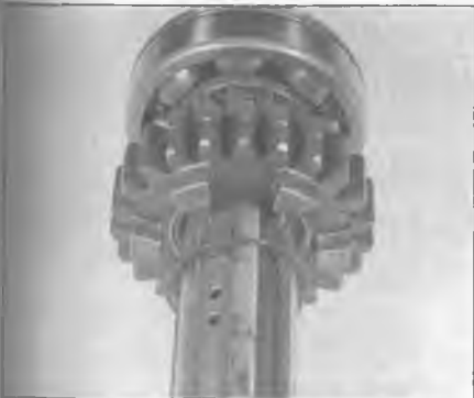
30.7b ... the toothed washer and fifth gear ...
