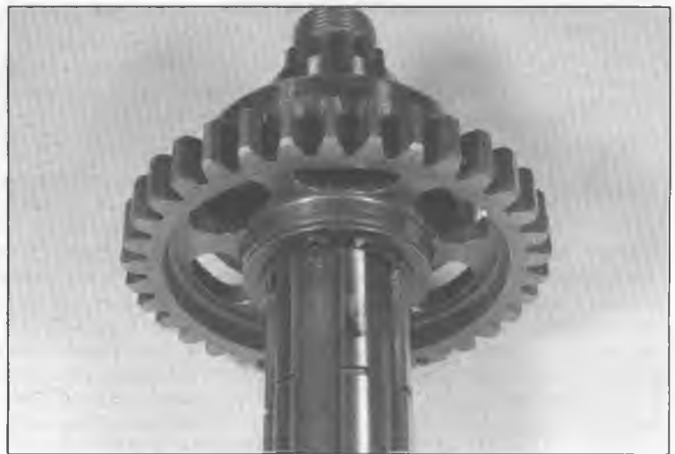
30.19a Remove the snap-ring ...
