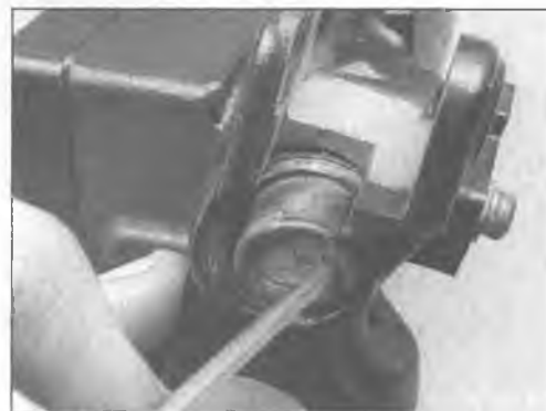
5.9b Remove the rubber boot from the end of the master cylinder piston . . .
