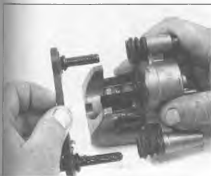
2.17c Pull the bracket out of the caliper . . .
