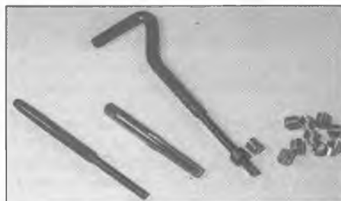
2.25 Obtain a thread insert kit to suit the thread diameter and pitch required
