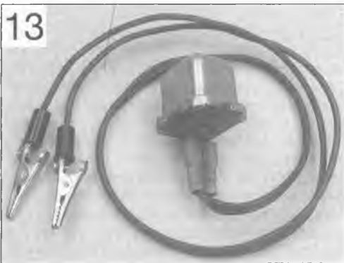
13 A buzzer is useful for voltage checks
