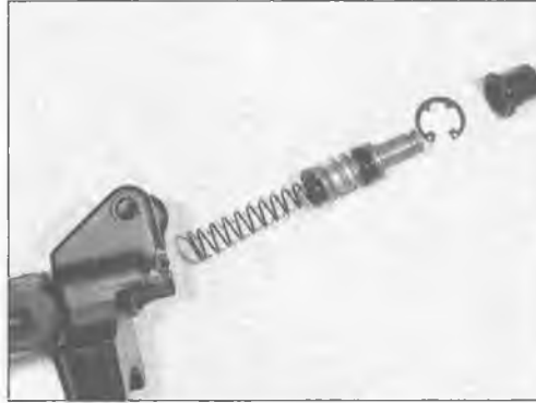
5.10b Lay out the old parts from the master cylinder to help install the new parts correctly
