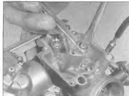
7.7 Prevent the needle jet holder from turning and unscrew the main jet with a screwdriver
