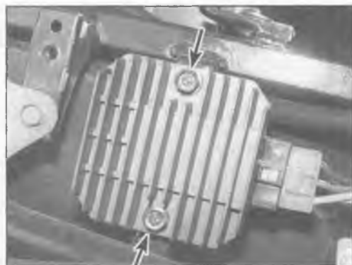
33.2 Simply remove these two bolts (arrows) and unplug the electrical connector
