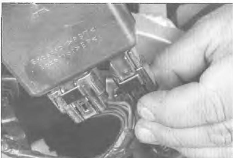
4.2b Unplug the pickup coil connector from the 2-pin connector located underneath the IC igniter (E models)
