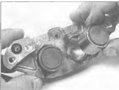
2.10 Remove the pistons from their bores
