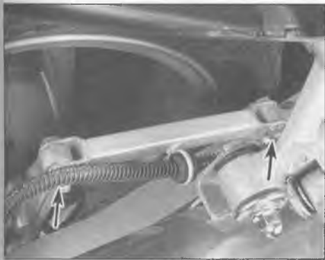
2.7 Before adjusting the chain, loosen both torque link nuts (arrows)
