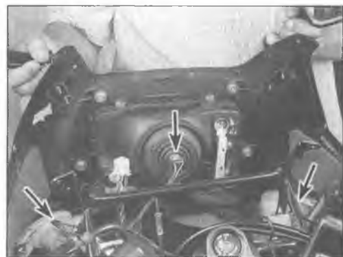
6.17 Unplug the electrical connectors for the headlight and turn signals (arrows) (E models)
