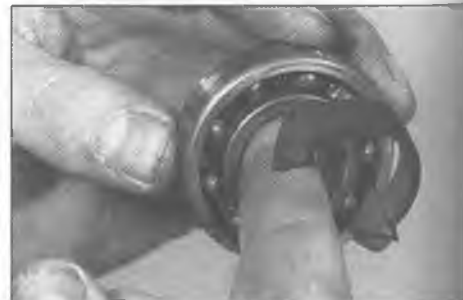
5.19 Hold outer race and listen to inner race when spun
