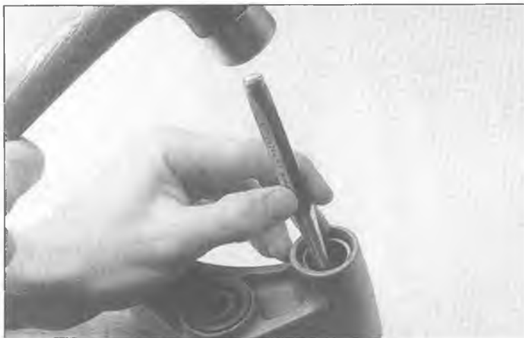
7.7 Knock out the old needle bearings with a hammer and punch
