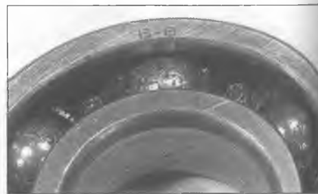
5.18 Example of ball journal bearing with damaged balls and cages
