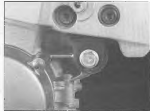
5.17b Remove the right front engine bolt, the Allen bolts above it and the right engine mounting bracket
