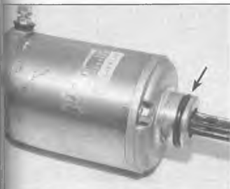
27.6 Inspect this O-ring on the starter; if it's cracked or torn, replace it
